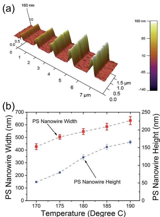
Fig. 2 (a) 3D AFM height image of PS NWs deposited using different temperatures but with the same tip speed of 150 nm s<sup>-1</sup>; (b) measured widths and heights of PS NWs deposited using different temperatures but with the same tip speed of 150 nm s<sup>-1</sup>.
