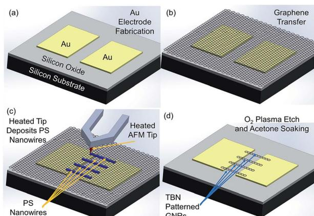
Fig. 1 Schematics illustrating major steps of GNR fabrication using TBN method with a heated AFM tip.
