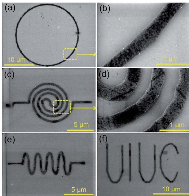
Fig. 4 SEM Images of different shapes of TBN-fabricated GNRs, demonstrating the fabrication flexibility of this TBN method. (a) A circular GNR with a radius of 10  $\mu\text{m}$ ; (b) a zoomed-in view of a section of the circular GNR; (c) a spiral-shaped GNR; (d) a zoomed-in view of a section of the spiral-shaped GNR; (e) a wavy-shaped GNR; (f) GNR forming the shape of "UIUC" representing University of Illinois at Urbana-Champaign.
