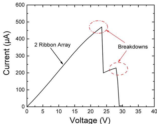
Fig. 8 Breakdown characteristics of 2 ribbon array. 2 breakdown levels are observed indicating the sequential breakdown of multiple ribbons. The calculated maximum current density is of the order of  $10^8$  A  $\text{cm}^{-2}$  which is consistent with literature-reported values.
