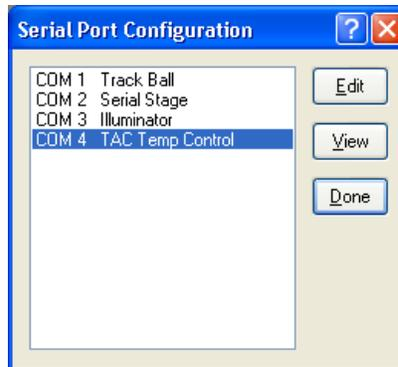
5. Highlight appropriate port and click **EDIT** in the **Serial Port Configuration** window to open the **Edit Port Setup** window, shown in [Figure 5.4f](#).
