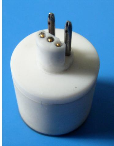
Two heater/cooler elements are required to cover the full temperature range,  $-35^{\circ}\text{C}$  to  $250^{\circ}\text{C}$ . Single experiments can be run from  $-35^{\circ}\text{C}$  to  $100^{\circ}\text{C}$  and from room temperature to  $250^{\circ}\text{C}$ .
