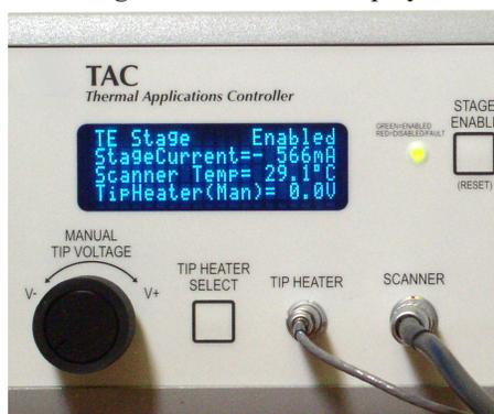
1. Heater type (**TE STAGE** - ThermoElectric heater/cooler, **HEAT STAGE** - High Temperature heater or **LOW T STAGE** — Air/Fluid heater — MultiMode only), **PID** parameters (air or fluid) and state (**ENABLED**, **DISABLED**, **ERROR**).
