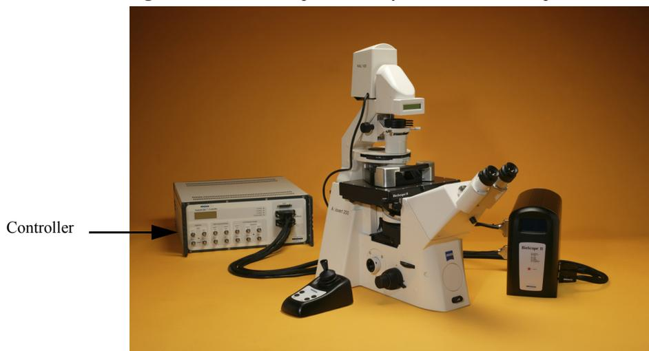
The NanoScope V functions with many advanced Bruker SPMs, including the MultiMode, MultiMode V, BioScope Catalyst, BioScope II, BioScope SZ, Dimension Icon, Dimension V, Dimension 5000 and EnviroScope atomic force microscopes (AFMs). The NanoScope V Controller is not compatible with the Dimension Metrology Head.
