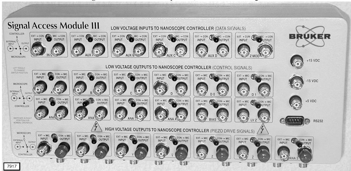
Figure 12.1c SAMIII: Side Panel, Access to Application Module Signals
