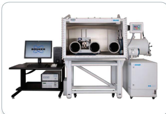
Figure 15. Turnkey glove-box enabling all AFM functions to be performed in a 1ppm level oxygen and water environment. Shown inside is a Dimension Icon AFM, a version of glove-box for the MultiMode 8 is also available.
