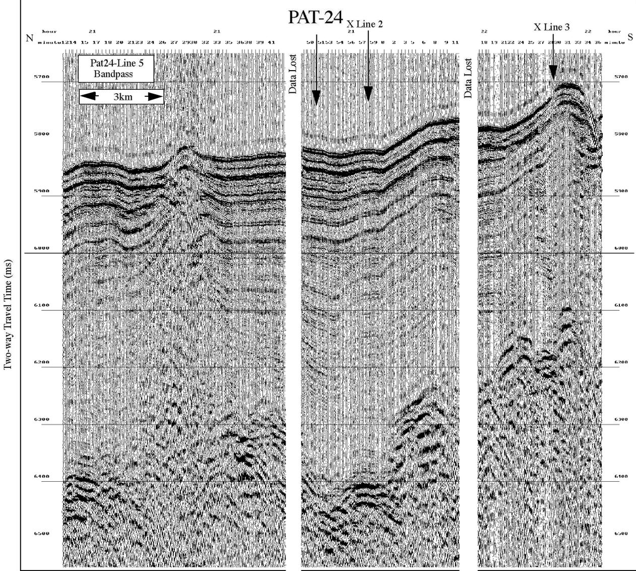
Figure PAT24-4: The 3.5 kHz profile PAT24-35line 5 across PAT-24, from EW9709
