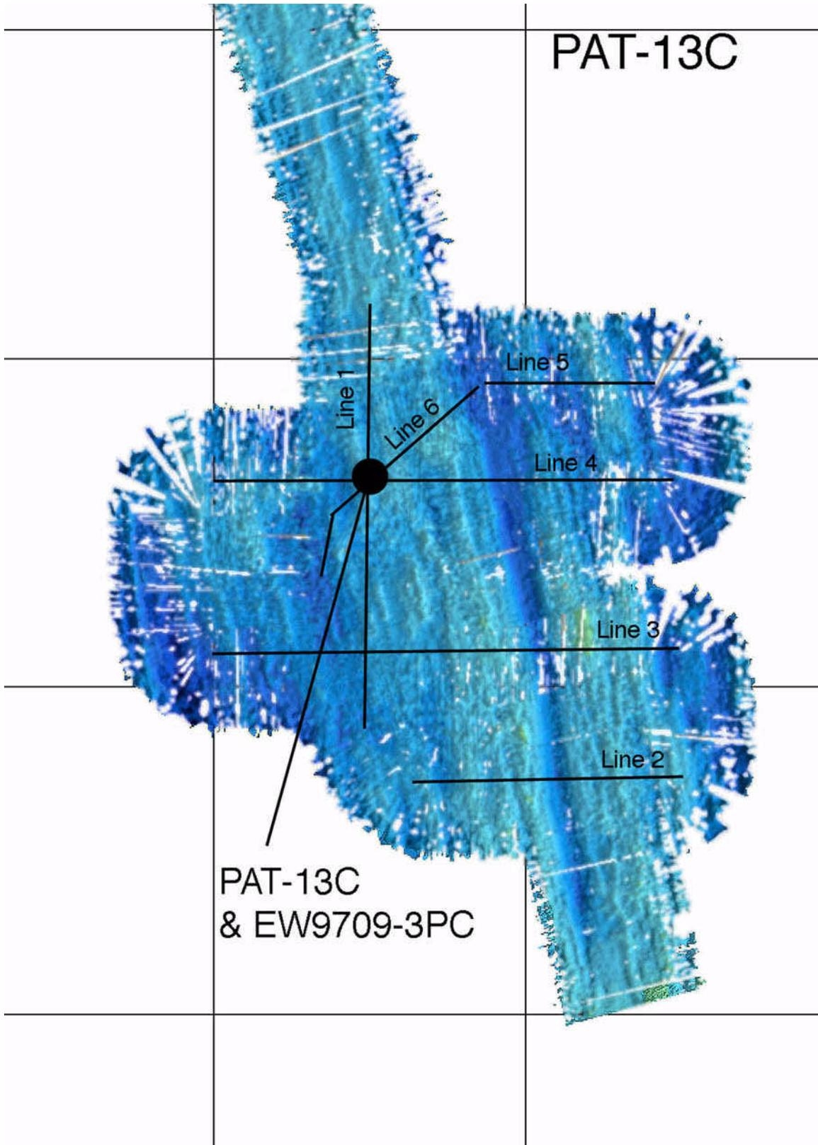
Figure PAT13-3: EW9709 PAT13-seisline4 showing proposed PAT-13C drillsite.
