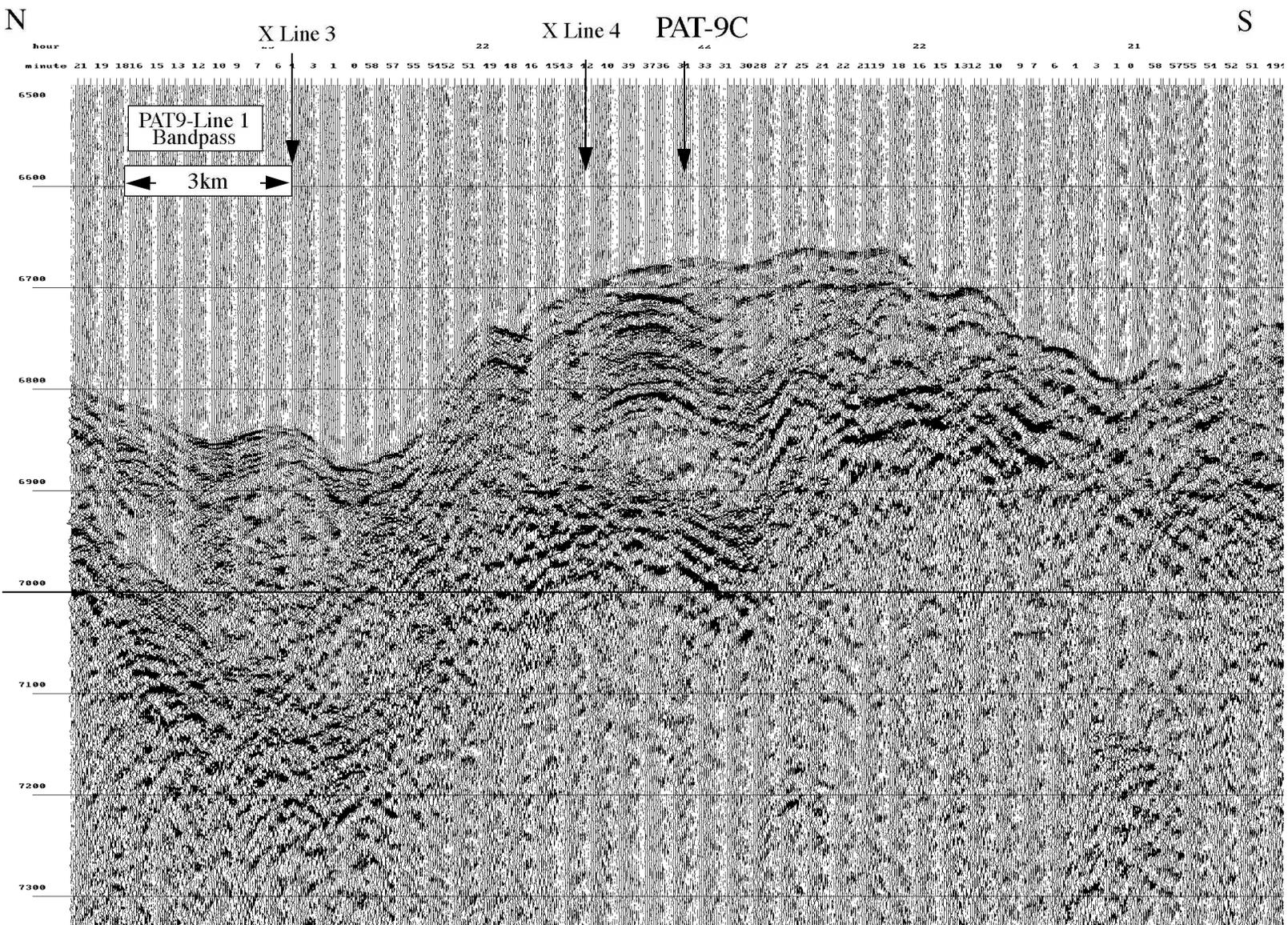
Figure PAT9-4: 3.5 KHz subbottom profile PAT9-35line 1 across PAT-9C, from FW9709.
