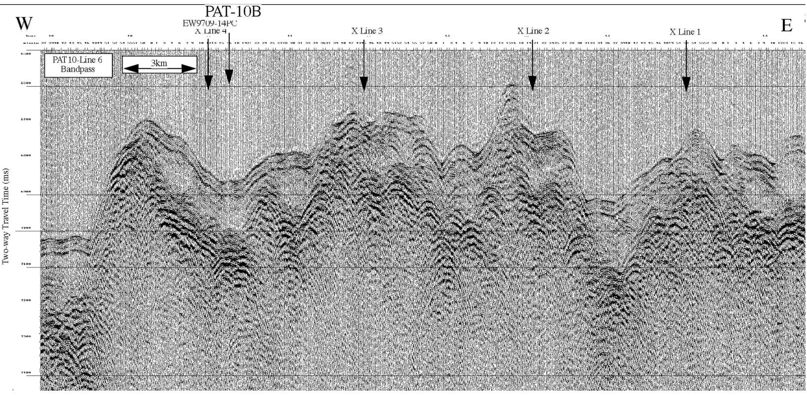
Fig PAT10-4: 3.5 kHz subbottom profile PAT10-35line 6 across PAT-10B, from EW9709. Proposed drill site is marked
