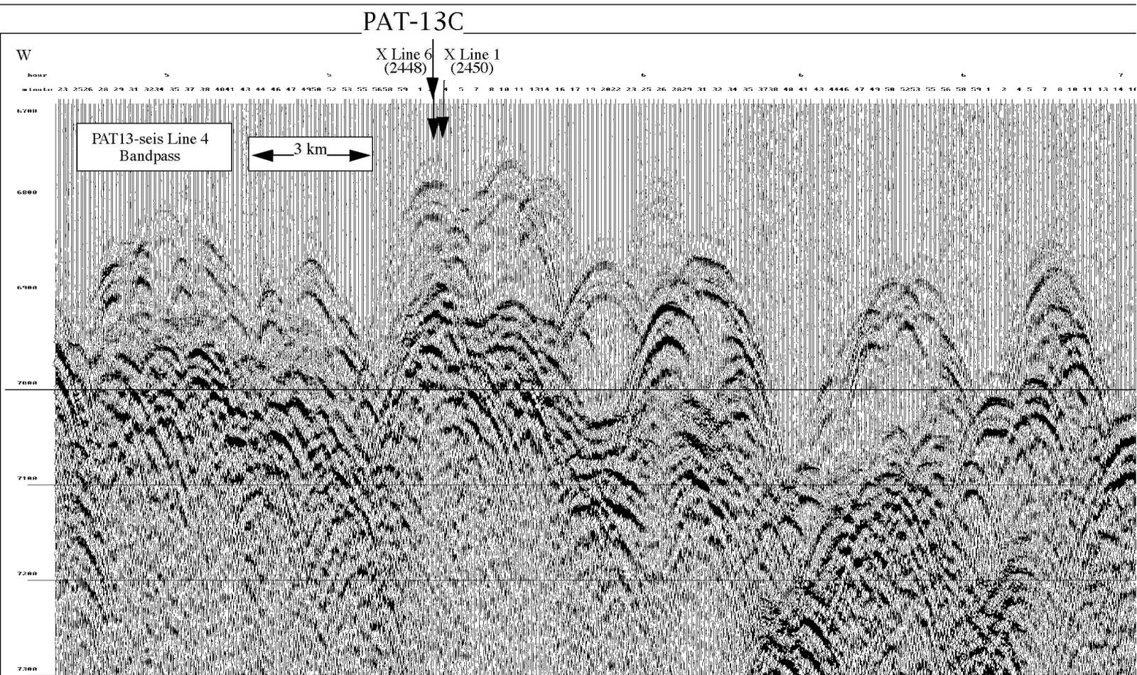
Figure PAT13-4: 3.5 kHz subbottom profile across PAT-13C (line PAT13-35line 4).
