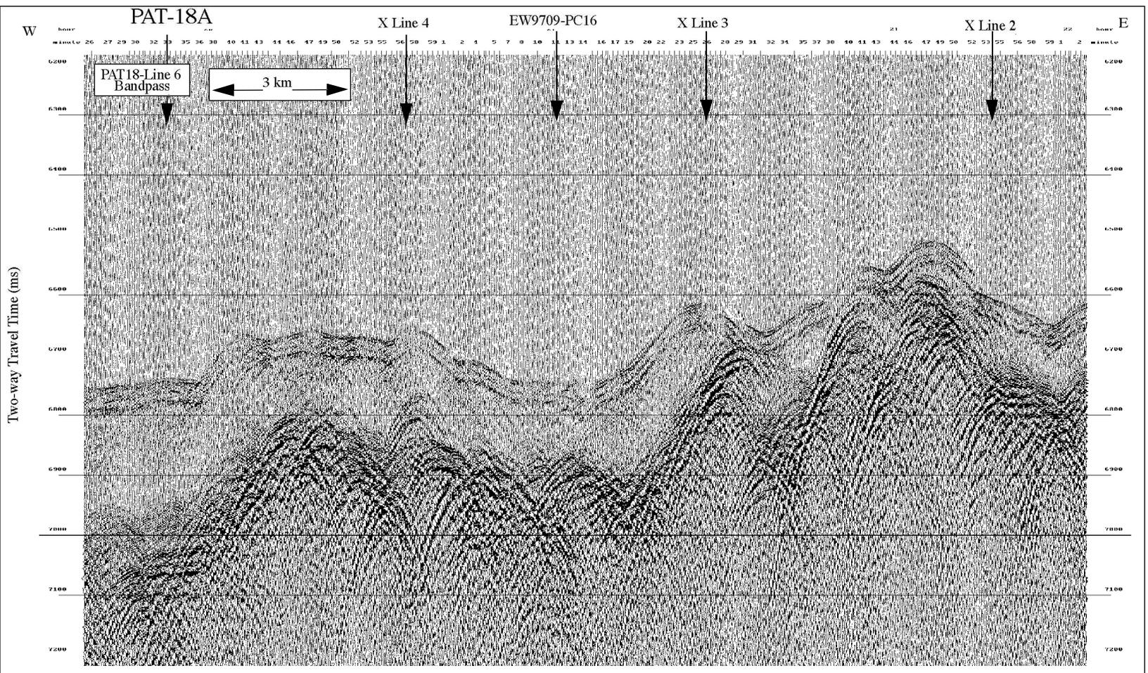
Figure PAT18-4: 3.5 kHz subbottom profile PAT18-35line 6 across PAT-18A
