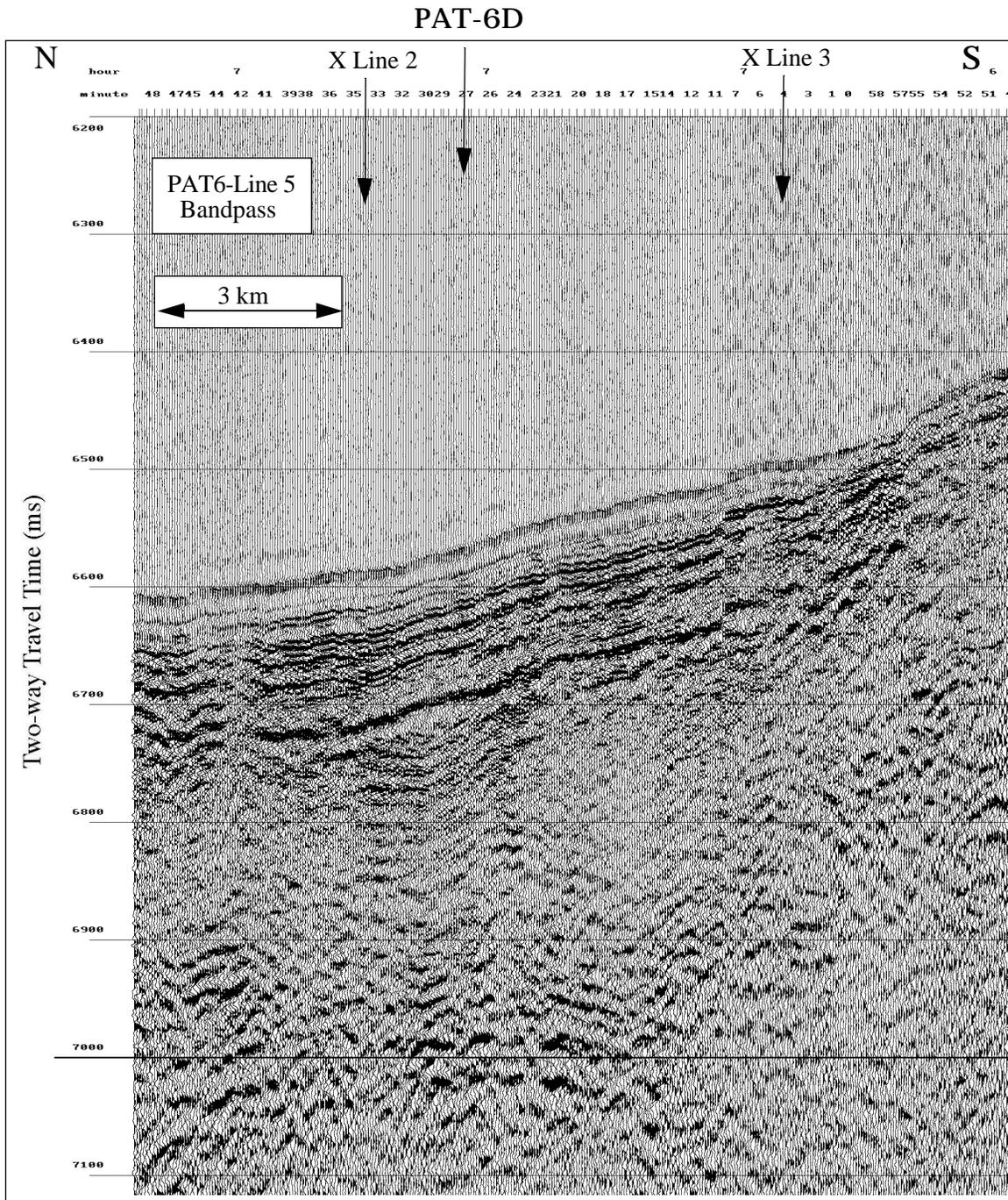
Figure PAT6-4: 3.5 kHz subbottom profile PAT6-35line 5 across PAT-6D, from EW9709.
