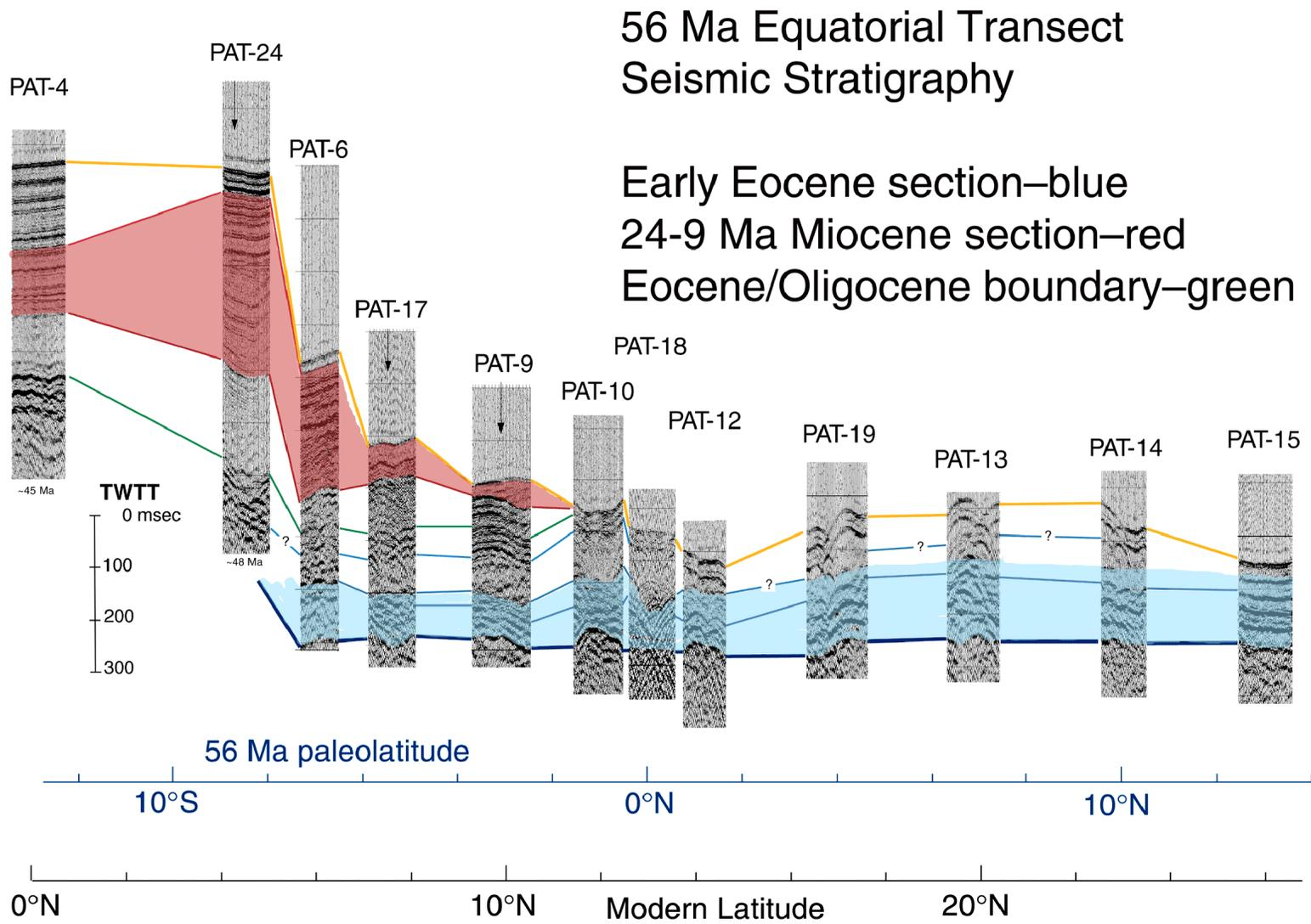
Figure Intro-2: Transect from the modern equator along the planned 56 Ma transect. All Priority 1 drillsites are shown as well as the Priority 2 sites PAT-24 and PAT-4B from the 40 Ma transect. The Miocene stratigraphy is based upon Mayer et al., 1985, constrained at the sediment surface by EW9709 piston cores. The Eocene seismic stratigraphy is based upon our best estimates but with no real age control.
