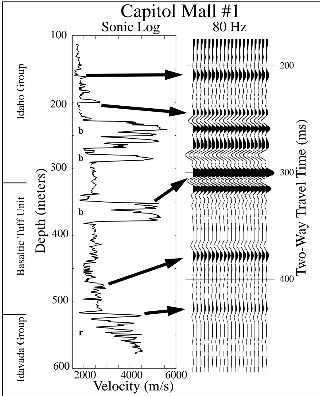
**FIGURE 13.** Sonic log from Capitol Mall #1 injection well with synthetic seismogram. The seismogram was calculated using an 80 Hz minimum phase Ormsby wavelet. Arrows point to the associated depth corrected times based on an RMS velocity model. High velocity layers are volcanic rocks: b=basalt, r=rhyolite.
