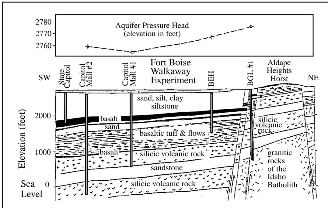
**FIGURE 10.** Geologic cross-section through downtown Boise based on local geothermal wells (from Burnham and Wood, 1985). The section has equal horizontal and vertical scales.
