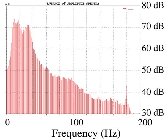
**FIGURE 8.** A comparison of kinestik vs. air gun sources at Ann Morrison Park. Both sources produced adequate energy to image the target zone. Spectral analysis plots are from the entire record lengths.
