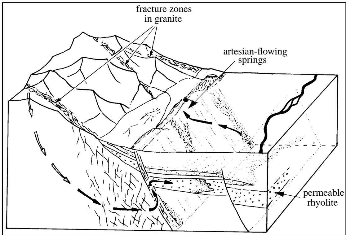
**FIGURE 3.** Conceptual model of the groundwater circulation system (from Wood and Burnham, 1987).
