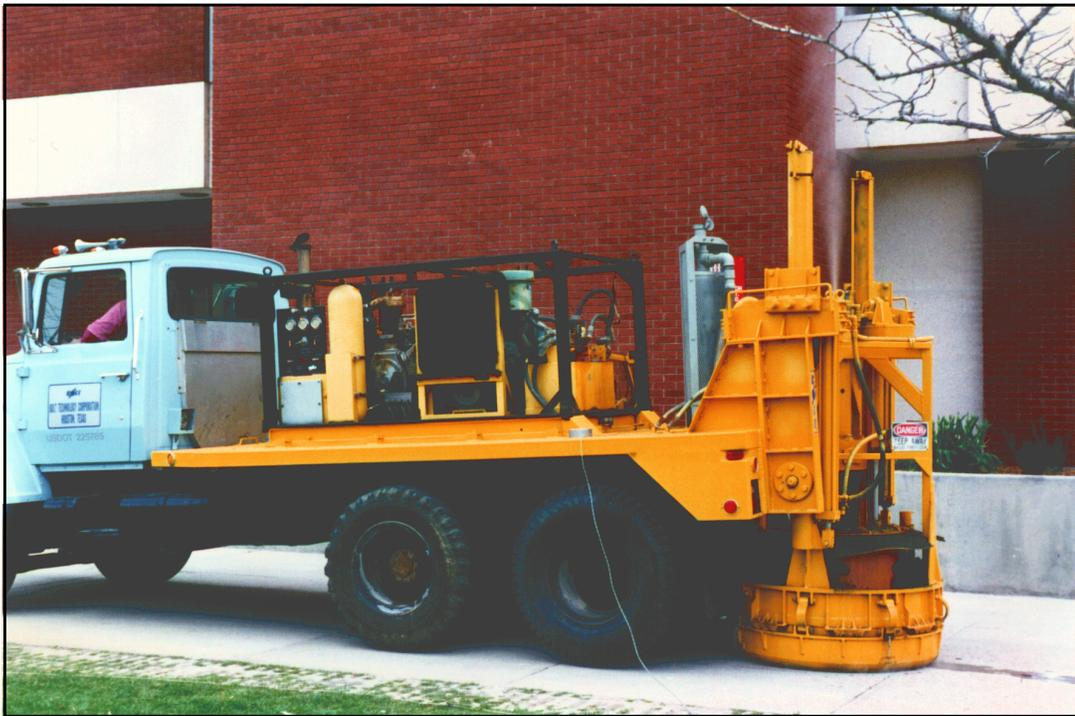
**FIGURE 4.** Airgun source used for the Boise geothermal seismic experiment. Distance from the building was approximately 5 m.
