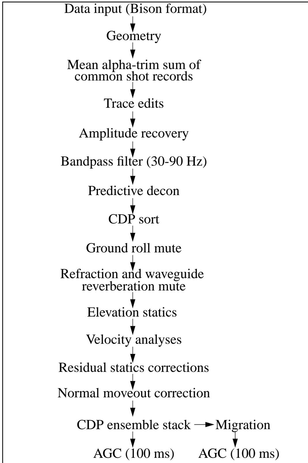
**FIGURE 11.** Processing flow chart for the Boise Geothermal seismic reflection data. Data were processed using Landmark's ProMAX seismic processing package.
