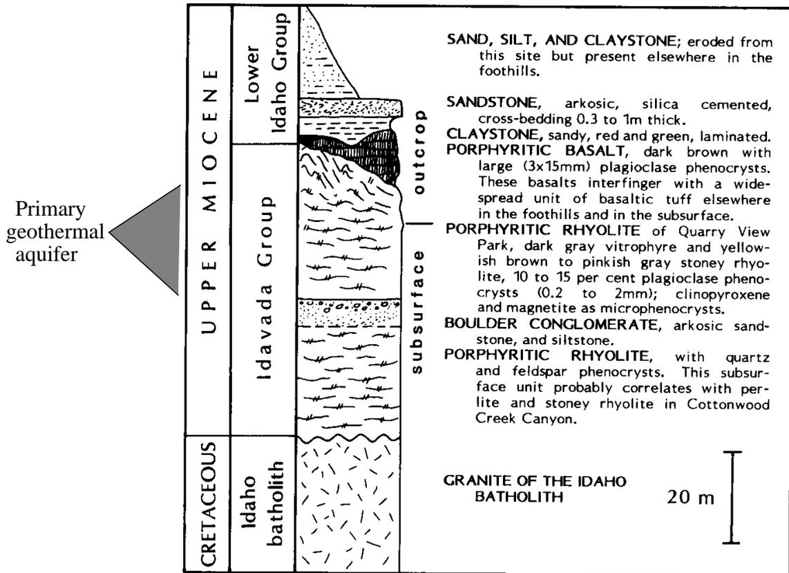
FIGURE 2. Stratigraphic section from rocks related to the geothermal system (from Wood and Burnham, 1987).
