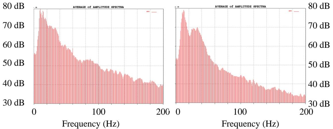
**FIGURE 9. A comparison of kinestik vs. air gun sources at Fort Boise Park. Both sources produced adequate energy to image the target zone. Spectral analysis plots are from the entire record lengths.**
