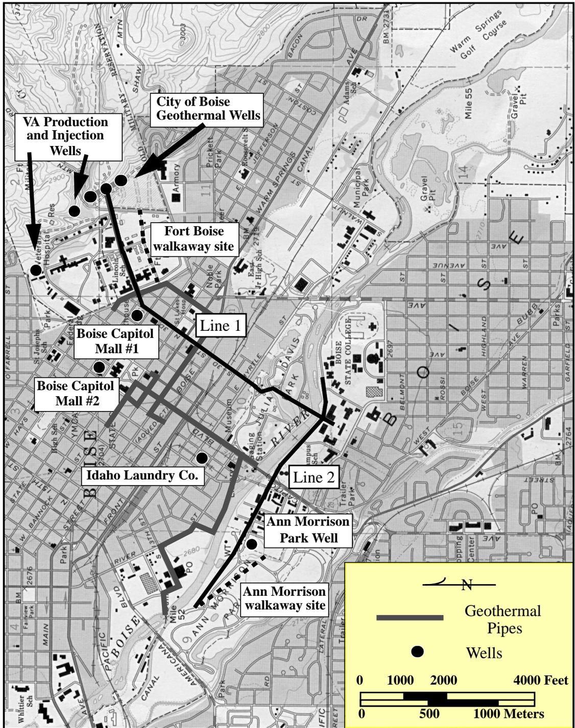
**FIGURE 1. Location map of downtown Boise, Idaho. Seismic reflection line locations, walkaway test sites, Boise City geothermal pipes and relevant wells are shown.**
