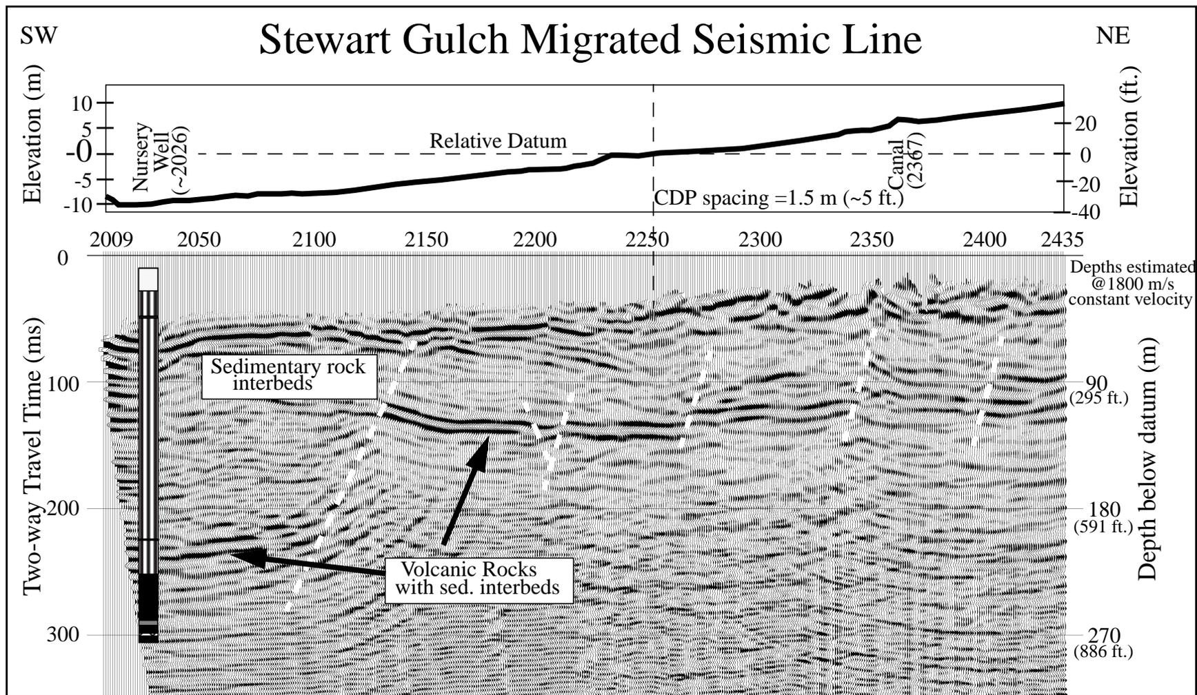
Figure 8. Migrated seismic reflection profile from the western half of the Stewart Gulch seismic line. The high-amplitude reflection package is interpreted to be due to the interface between near-surface sedimentary rocks and deeper volcanic rocks assemblage (from the Nursery well lithologic log). The section is plotted with no vertical exaggeration and well log patterns are described in Figure 4. Note the coherent “smile” artifacts from the migration process.
