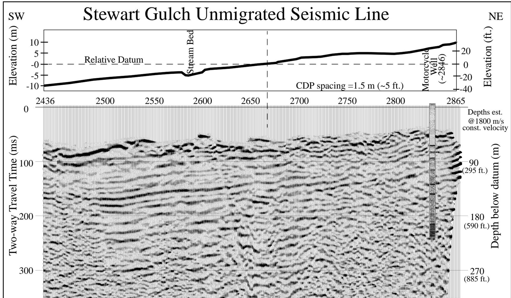
Figure 7. Seismic reflection profile from the eastern half of the Stewart Gulch line. The datum crosses the line at CDP 2667. The datum for elevation statics is 38 ms less than the datum on Figure 6. The section is plotted with no vertical exaggeration and well log patterns are described in Figure 4.
