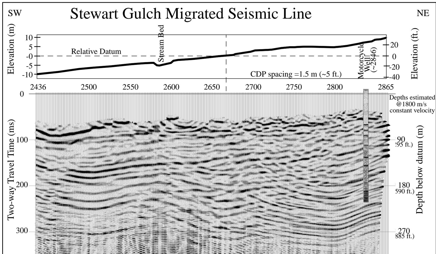
Figure 9. Migrated seismic reflection profile from the eastern half of the Stewart Gulch line. The lithologic log from the Motorcycle well is projected on the section. The datum crosses the line at CDP 2667. The section is plotted with no vertical exaggeration and well log patterns are described in Figure 4. Note the coherent “smile” artifacts from the migration process.
