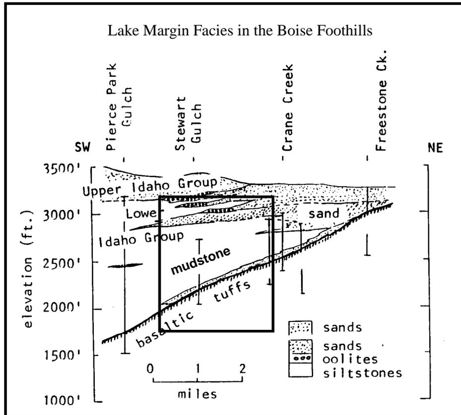
Figure 2. Cross-section depicting the shallow stratigraphy near Stewart Gulch in the Boise foothills (box shows field site location). Elevations near the seismic lines vary from 2800 to 3100 ft. Figure modified from Gallegos and others (1987).
