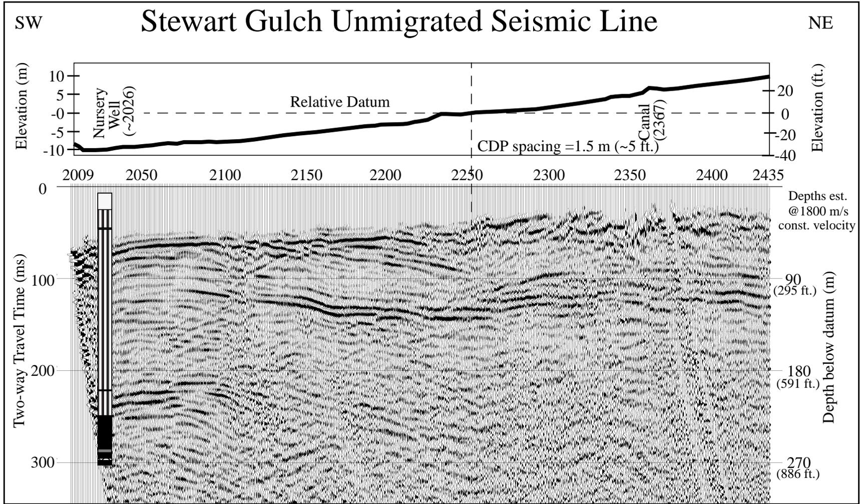
Figure 6. Seismic reflection profile from the western half of the Stewart Gulch seismic line. The datum crosses the profile at CDP 2255. The section is plotted with no vertical exaggeration and well log patterns are described in Figure 4.
