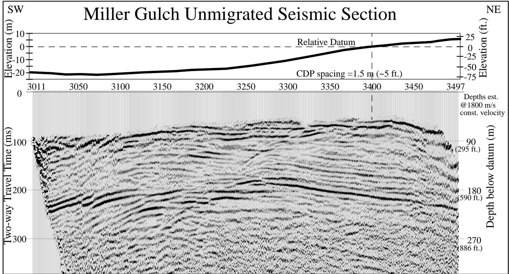
Figure 10. Unmigrated seismic reflection profile from Miller Gulch. Note the strong reflection package from 190-230 ms TWTT. There is no well control in the region. The section is plotted with no vertical exaggeration.
