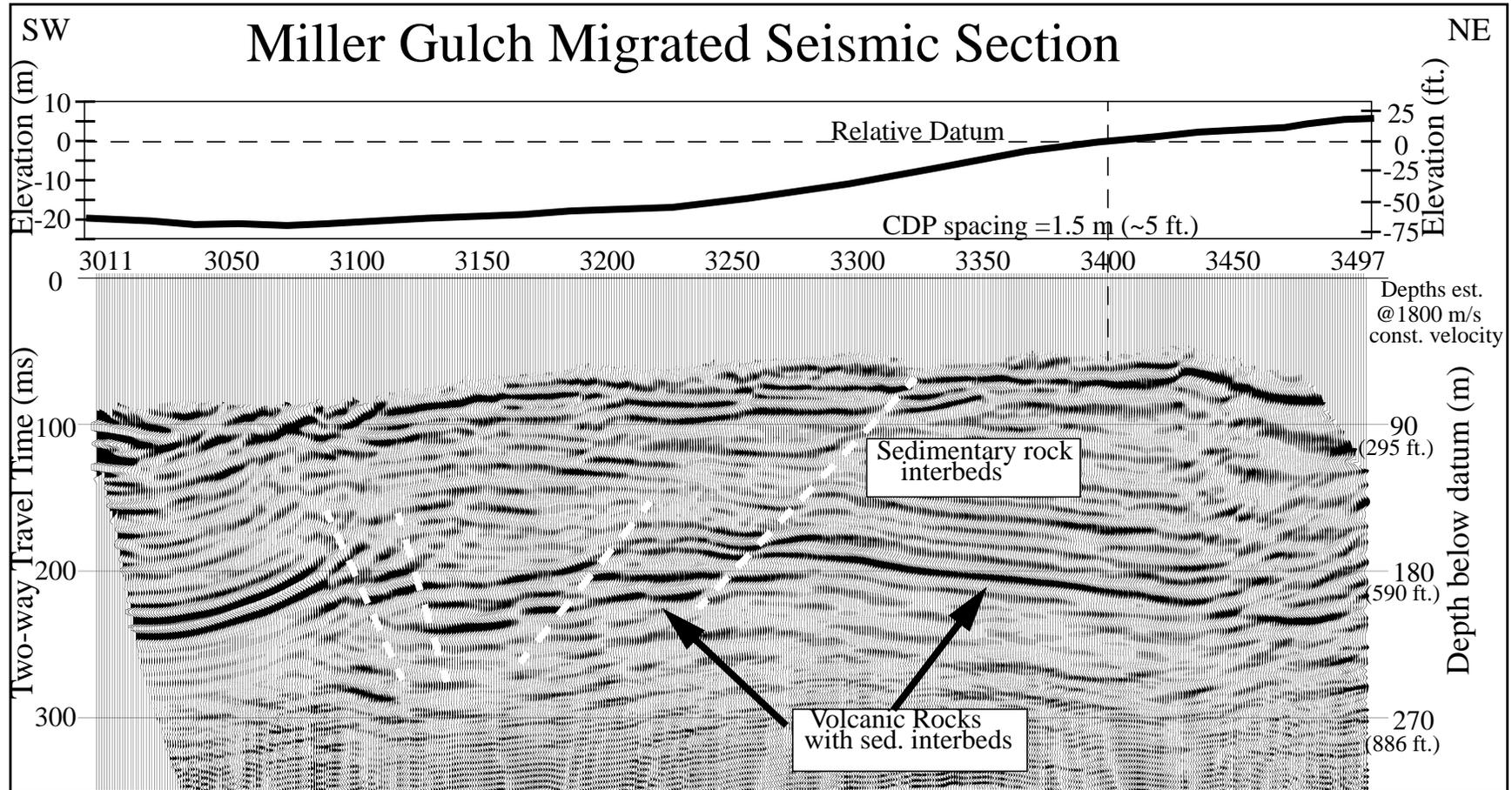
Figure 11. Migrated seismic reflection profile from Miller Gulch. The high-amplitude reflection package is interpreted as the interface between interbedded sedimentary rocks and a volcanic rock assemblage. This interpretation is based on an extrapolation of the geology from the Stewart Gulch and Airstrip seismic lines. The section is plotted with no vertical exaggeration. Note the coherent "smile" artifacts from the migration process.
