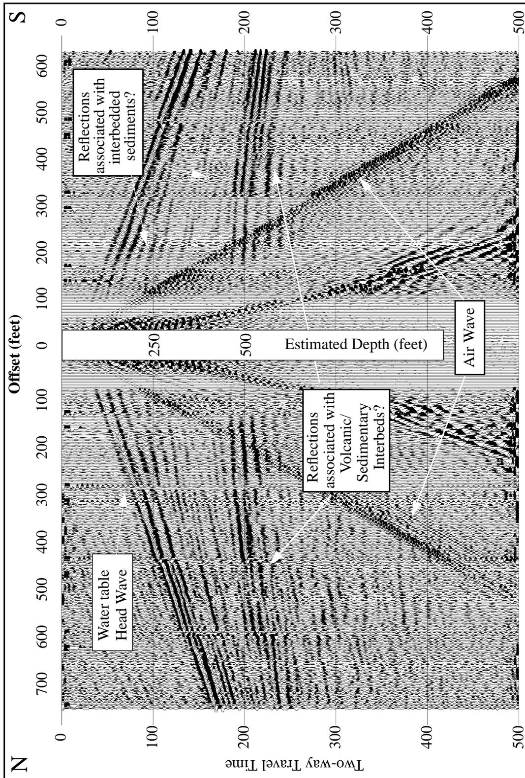
**Figure 4.** EWG walkaway results from the Windsock well location. The high quality of the walkaway results from the saturated near-surface conditions, minor topography and uniform lateral geology.
