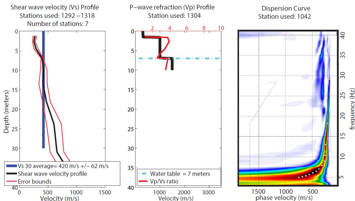
**Figure 5. (left) Shear wave velocity profile and average Vs30 calculation for the central portion of the Forest Road profile. (middle) P-wave, Vp/Vs ratio and water table depth measurement for the central portion of the profile. (right) Shot gather derived dispersion curve and phase velocity picks suggesting high confidence results for the upper 40 m.**
