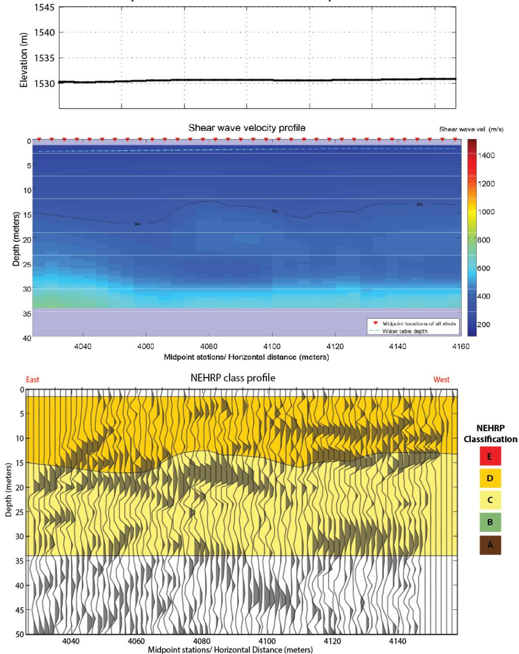
Figure 12. (top) Elevation profile for the Lenora Street profile. (middle) Shear wave velocity profile derived from phase velocity picks. Measurement locations are show as red triangles at the top of the plot. Semi-transparent area represents low confidence zones. (bottom) NEHRP class profile with superposition of reflection image. Velocity profile vertical exaggeration ~1:1.
