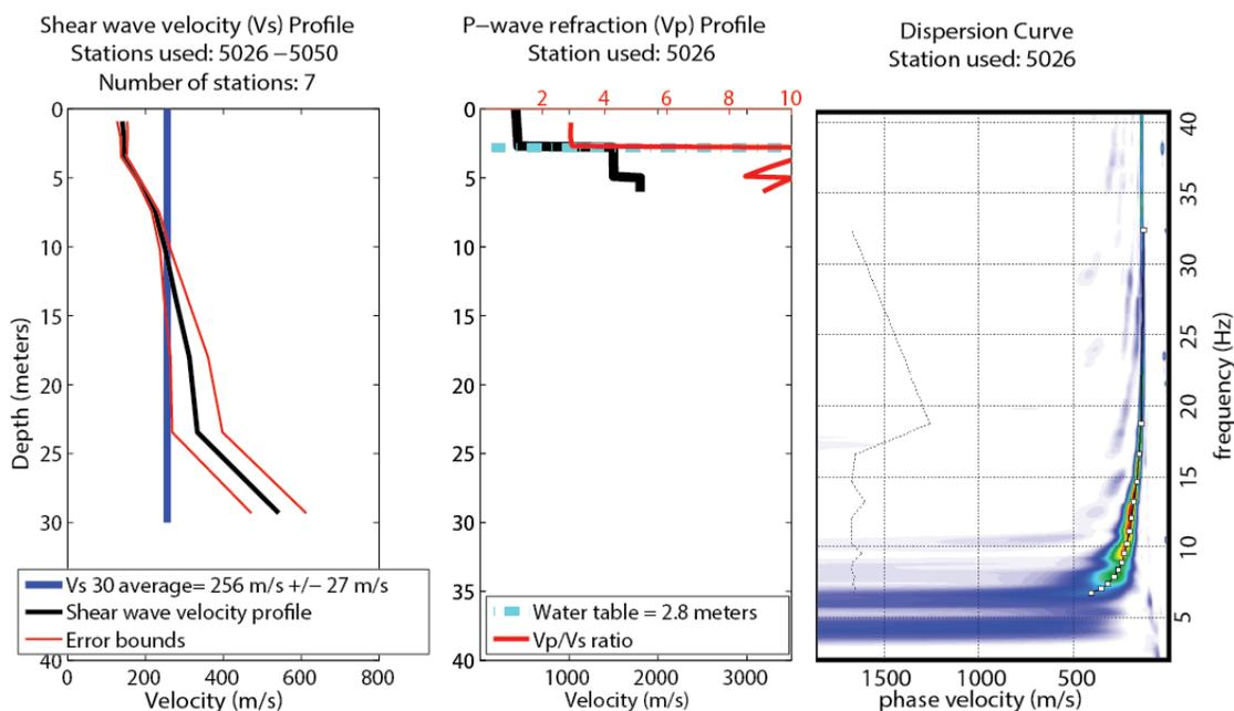
**Figure 46.** (left) Shear wave velocity profile and average  $V_{S30}$  calculation for the Sewage (city Park) profile. (middle) P-wave,  $V_p/V_s$  ratio and water table depth measurement for the central portion of the profile. (right) Shot gather derived dispersion curve and phase velocity picks suggesting high confidence results for the upper 30 m.
