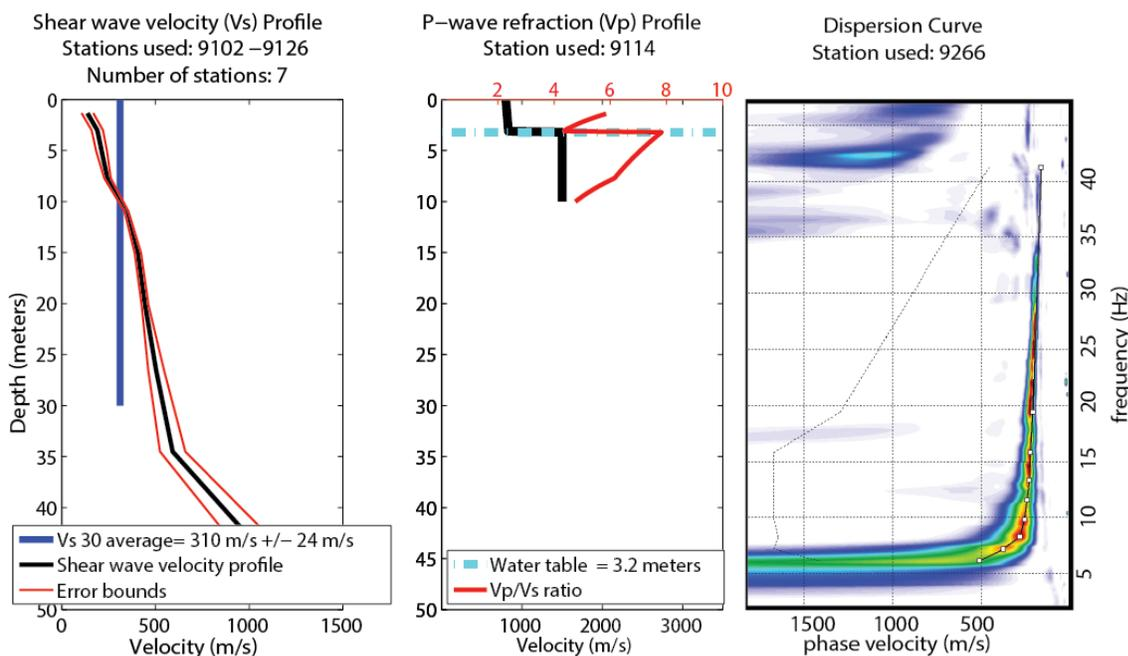
**Figure 21.** (left) Shear wave velocity profile and average  $V_{S30}$  calculation for the central portion of the Mill Road profile. (middle) P-wave,  $V_p/V_s$  ratio and water table depth measurement for the central portion of the profile. (right) Shot gather derived dispersion curve and phase velocity picks suggesting high confidence results for the upper 42 m.
