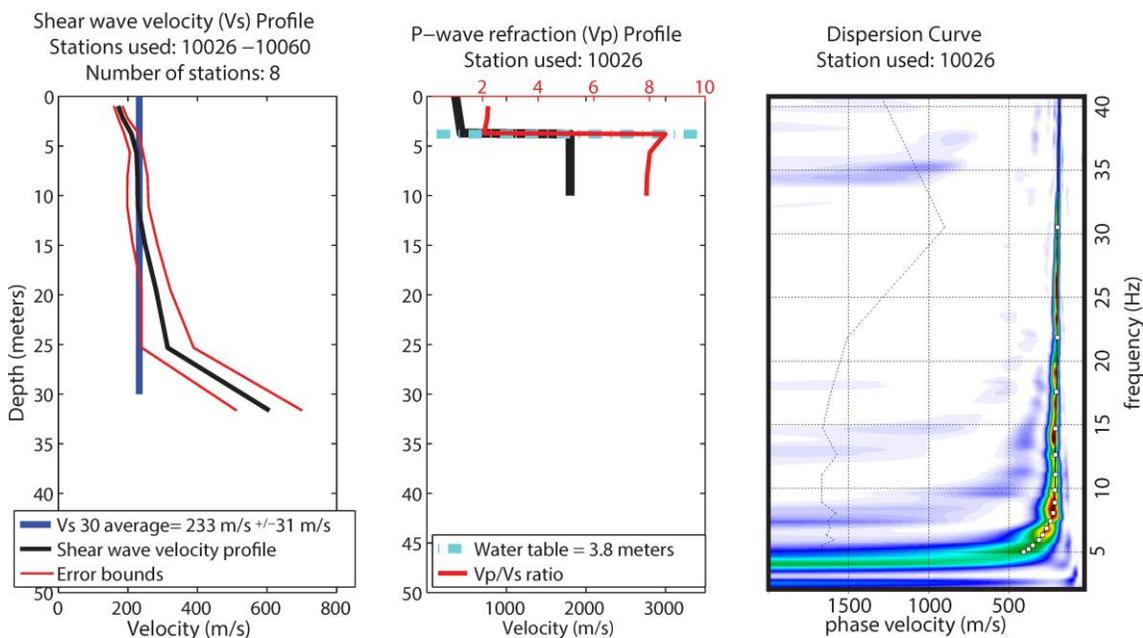
**Figure 25. (left) Shear wave velocity profile and average VS30 calculation for the central portion of the RV Park access road profile. (middle) P-wave, Vp/Vs ratio and water table depth measurement for the central portion of the profile. (right) Shot gather derived dispersion curve and phase velocity picks suggesting high confidence results for the upper 32 m.**
