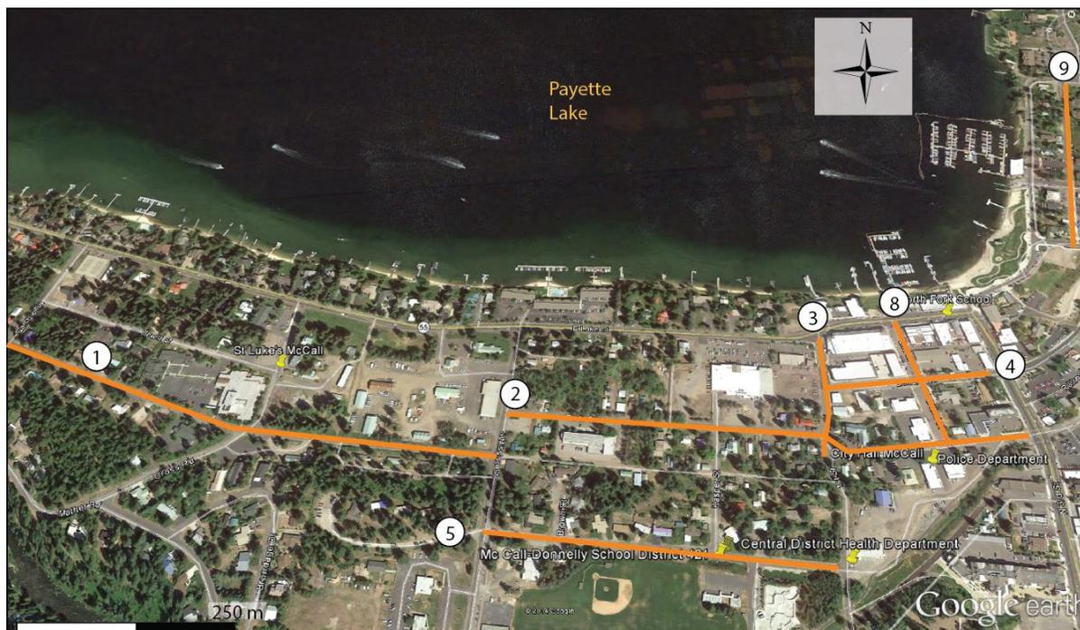
**Figure 4. Downtown McCall aerial photo with seismic profile locations.**
