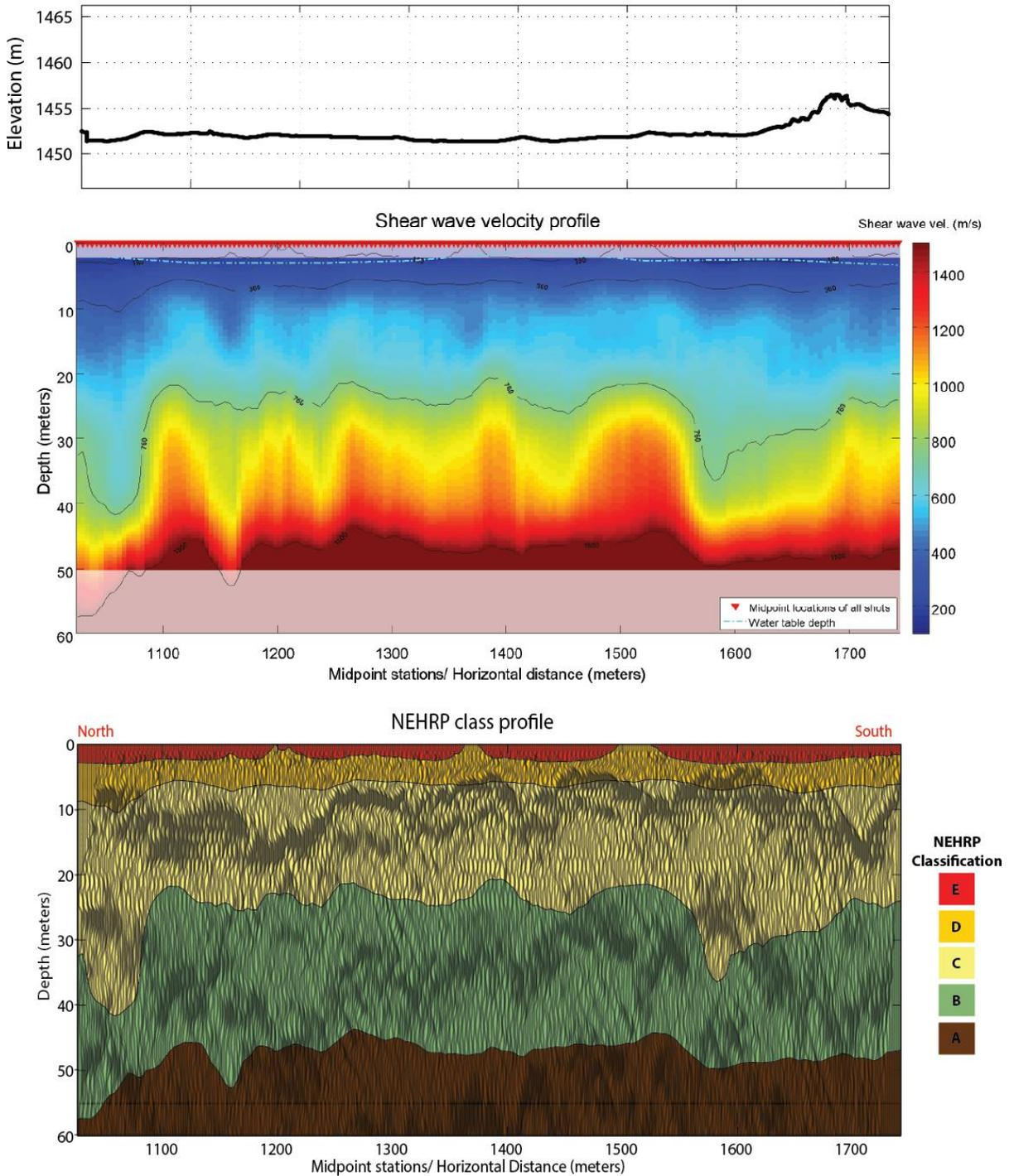
Figure 39. (top) Elevation profile for the Idaho Street profile. (middle) Shear wave velocity profile derived from phase velocity picks. Measurement locations are show as red triangles at the top of the plot. Semi-transparent area represents low confidence zones. (bottom) NEHRP class profile with superposition of reflection image. Velocity profile vertical exaggeration ~4:1.
