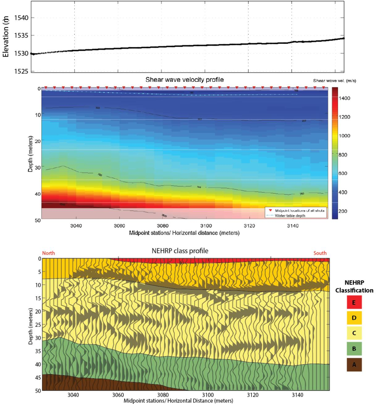
Figure 10. (top) Elevation profile for the First Street profile. (middle) Shear wave velocity profile derived from phase velocity picks. Measurement locations are show as red triangles at the top of the plot. Semi-transparent area represents low confidence zones. (bottom) NEHRP class profile with superposition of reflection image. Velocity profile vertical exaggeration ~1:1.
