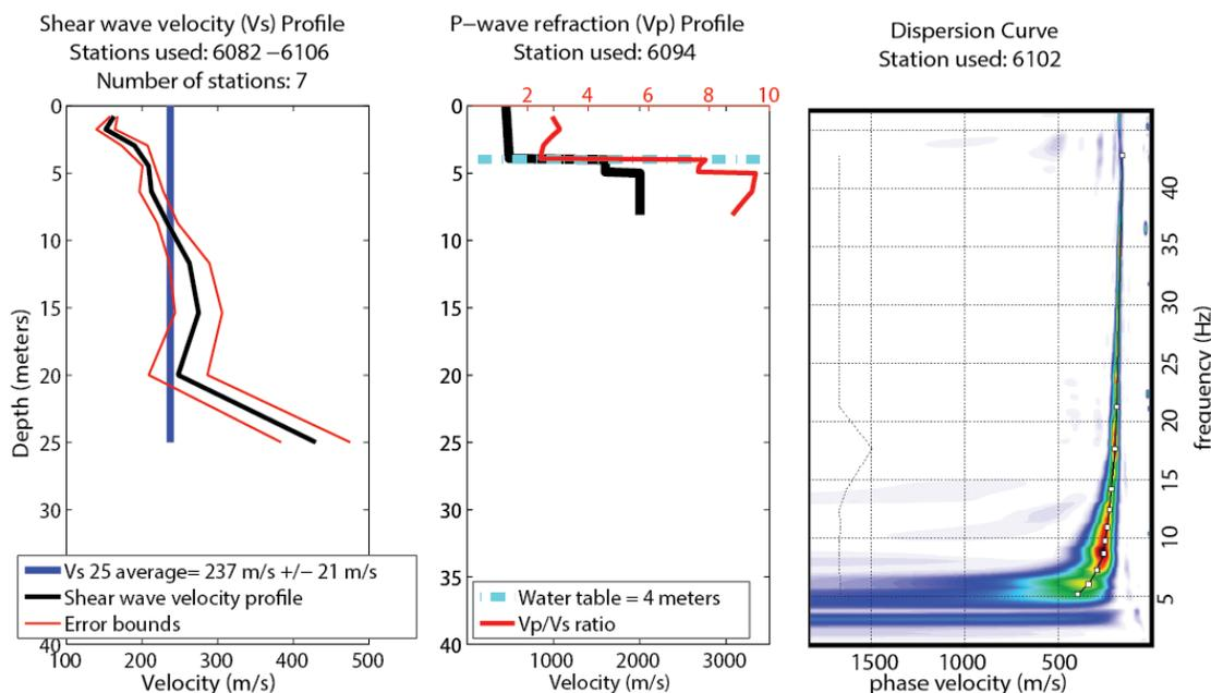
**Figure 48. (left) Shear wave velocity profile and average VS30 calculation for the central portion of the Alzar profile. (middle) P-wave, Vp/Vs ratio and water table depth measurement for the central portion of the profile. (right) Shot gather derived dispersion curve and phase velocity picks suggesting high confidence results for the upper 25 m.**
