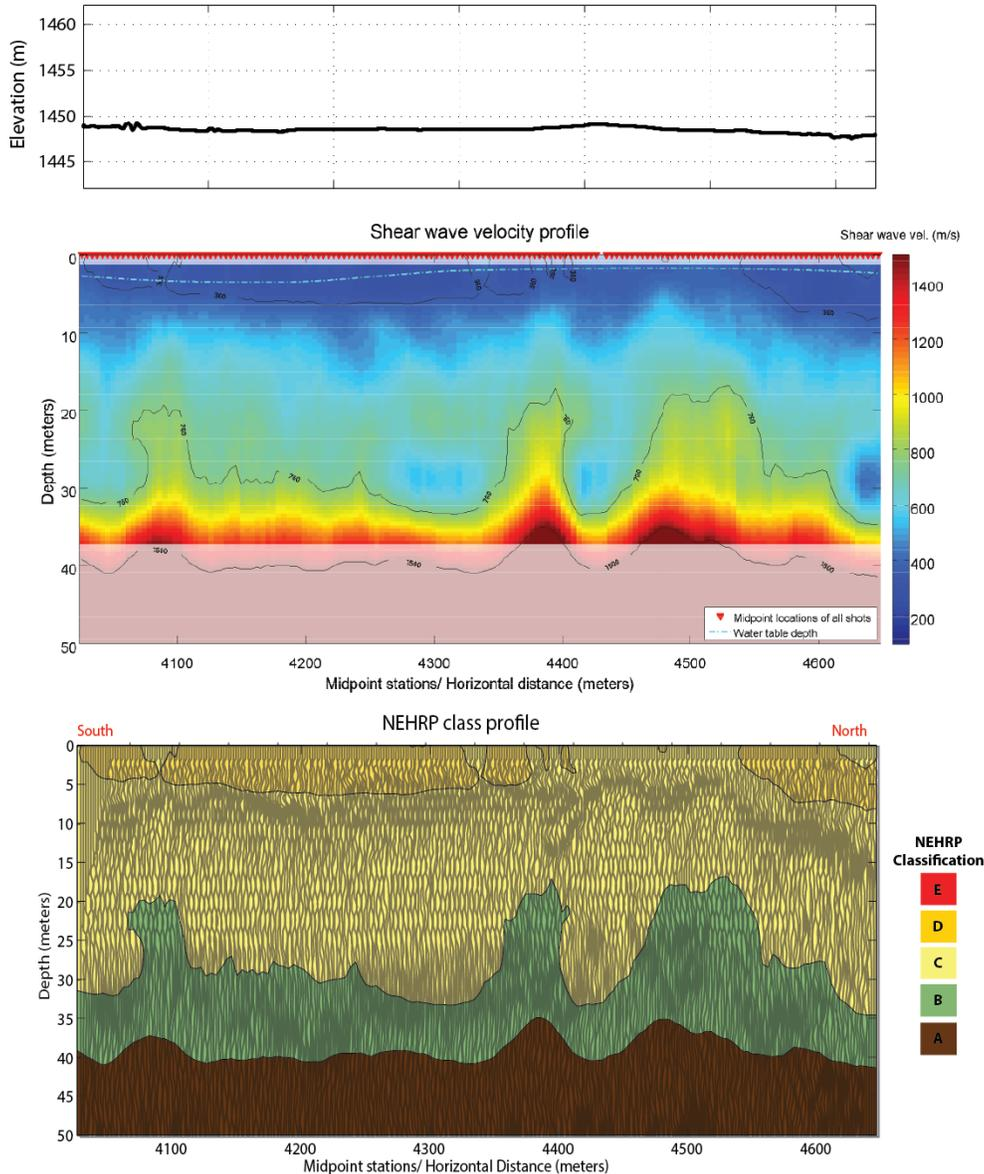
**Figure 45. (top) Elevation profile for the Forest Street profile. (middle) Shear wave velocity profile derived from phase velocity picks. Measurement locations are show as red triangles at the top of the plot. Semi-transparent area represents low confidence zones. (bottom) NEHRP class profile with superposition of reflection image. Velocity profile vertical exaggeration ~5:1.**
