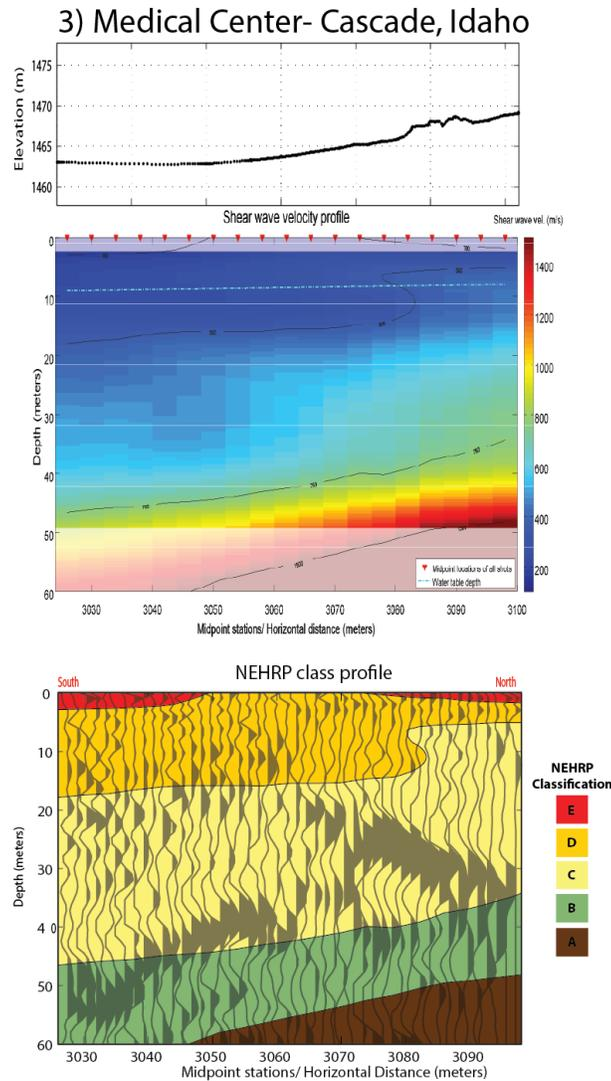
**Figure 43. (top) Elevation profile for Lefever Drive (Medical Center) profile. (middle) Shear wave velocity profile derived from phase velocity picks. Measurement locations are show as red triangles at the top of the plot. Semi-transparent area represents low confidence zone. (bottom) NEHRP class profile with superposition of reflection image. Velocity profile vertical exaggeration ~2:1.**
