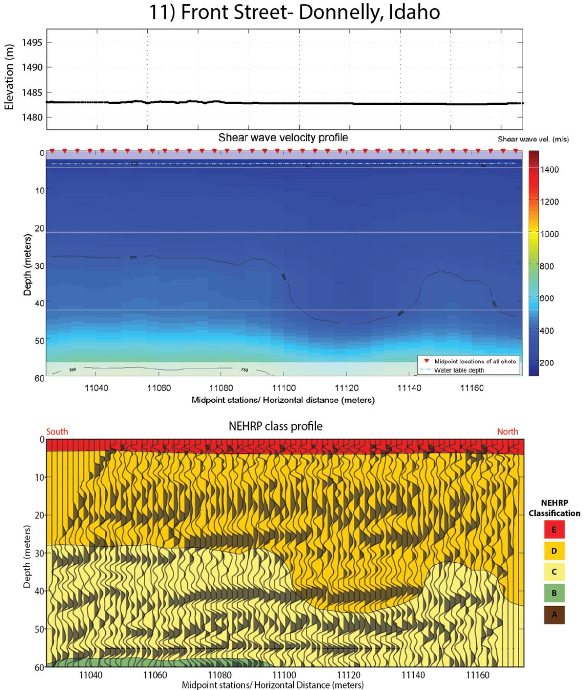
**Figure 30. (top) Elevation profile for the Front Street profile. (middle) Shear wave velocity profile derived from phase velocity picks. Measurement locations are show as red triangles at the top of the plot. Semi-transparent area represents low confidence zones. (bottom) NEHRP class profile with superposition of reflection image. Velocity profile vertical exaggeration ~1:1.**
