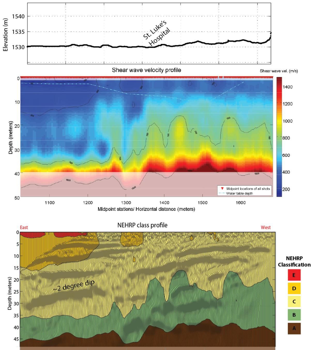
Figure 6. (top) Elevation profile for the Forest Street profile. (middle) Shear wave velocity profile derived from phase velocity picks. Measurement locations are show as red triangles at the top of the plot. Semi-transparent area represents low confidence zones. (bottom) NEHRP class profile with superposition of reflection image. Velocity profile vertical exaggeration ~6:1.
