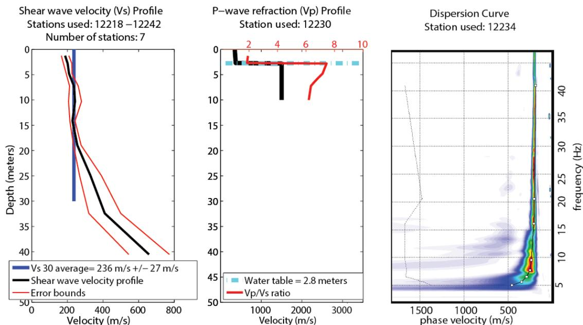
**Figure 33. (left) Shear wave velocity profile and average VS30 calculation for the central portion of the Halferty Street profile. (middle) P-wave, Vp/Vs ratio and water table depth measurement for the central portion of the profile. (right) Shot gather derived dispersion curve and phase velocity picks suggesting high confidence results for the upper 40 m.**
