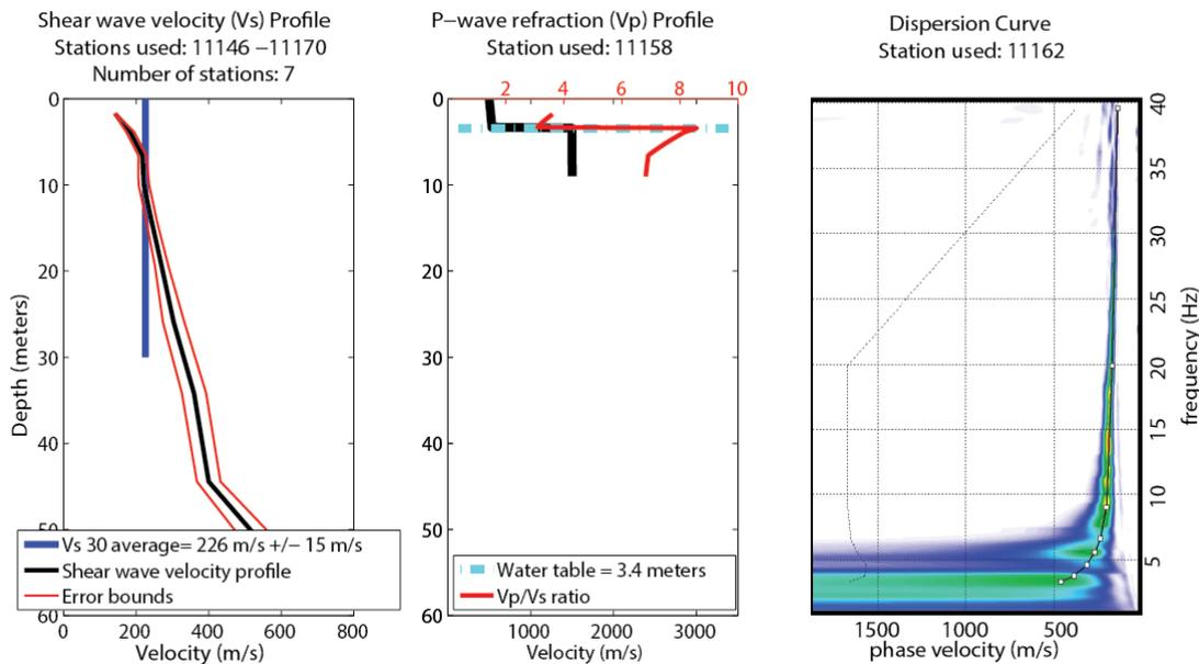
Figure 29. (left) Shear wave velocity profile and average VS30 calculation for the central portion of the Front Street profile. (middle) P-wave, Vp/Vs ratio and water table depth measurement for the central portion of the profile. (right) Shot gather derived dispersion curve and phase velocity picks suggesting high confidence results for the upper 58 m.
