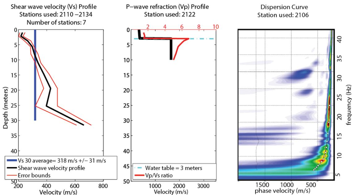
**Figure 8.** Shear wave velocity profile and average Vs30 calculation for the central portion of the Park Street profile. (middle) P-wave, Vp/Vs ratio and water table depth measurement for the central portion of the profile. (right) Shot gather derived dispersion curve and phase velocity picks suggesting high confidence results for the upper 32 m.
