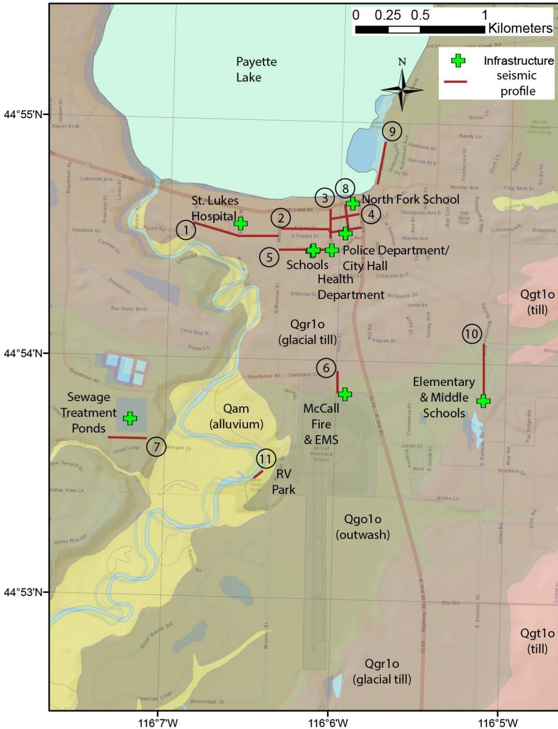
Figure 3. Seismic profile locations (red lines) for the McCall, Idaho area. The profile locations focused on critical infrastructure located within city limits. The circled numbers represent profile locations that are described below. Surficial geology from Breckenridge and Othberg (2006).
