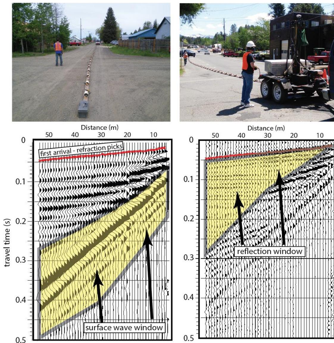
**Figure 1. (top) Seismic land streamer with seismic accelerated weight drop source during acquisition in Donnelly and McCall. (Bottom) Seismic shot gather unfiltered (left) and filtered (right) to emphasize first arrival picks (red stars), reflections, and surface waves.**
