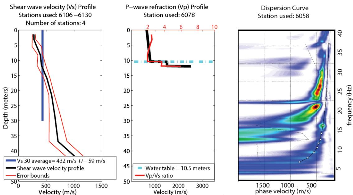
**Figure 15 (left) Shear wave velocity profile and average VS30 calculation for the central portion of the Thula Street profile. (middle) P-wave,  $V_p/V_s$  ratio and water table depth measurement for the central portion of the profile. (right) Shot gather derived dispersion curve and phase velocity picks suggesting high confidence results for the upper 32 m.**
