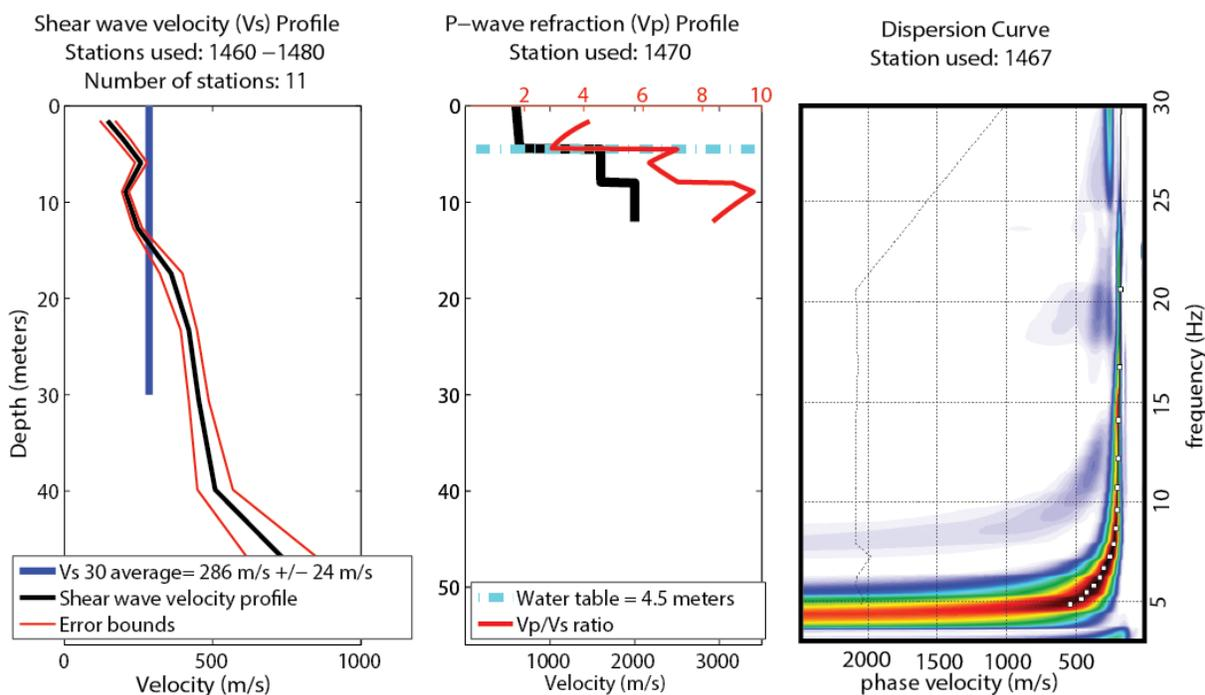
**Figure 50. (left) Shear wave velocity profile and average VS30 calculation for the central portion of the Stonebreaker profile. (middle) P-wave, Vp/Vs ratio and water table depth measurement for the central portion of the profile. (right) Shot gather derived dispersion curve and phase velocity picks suggesting high confidence results for the upper 25 m.**
