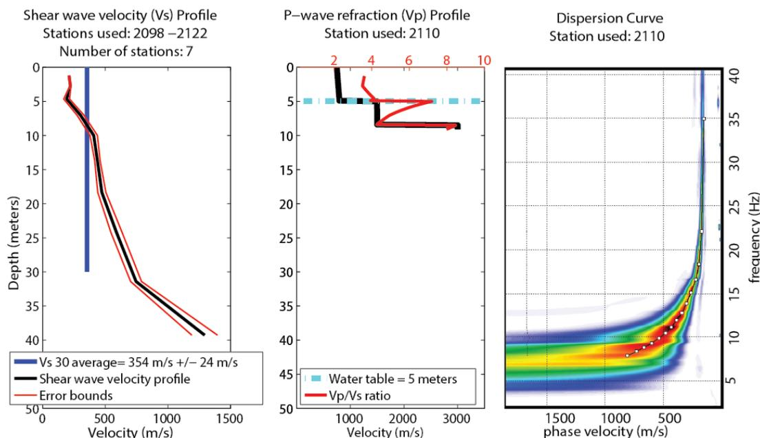
**Figure 40.** (left) Shear wave velocity profile and average  $V_{S30}$  calculation for the central portion of the Spring Street profile. (middle) P-wave,  $V_p/V_s$  ratio and water table depth measurement for the central portion of the profile. (right) Shot gather derived dispersion curve and phase velocity picks suggesting high confidence results for the upper 39 m.
