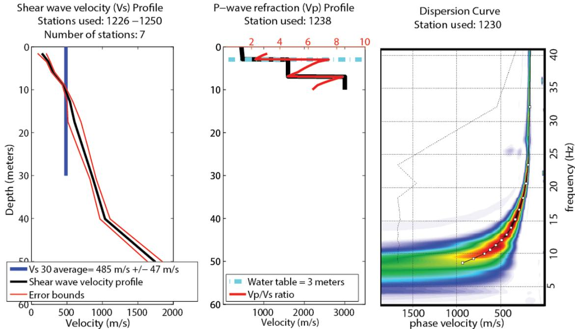
**Figure 38. (left) Shear wave velocity profile and average VS30 calculation for the central portion of the Idaho Street profile. (middle) P-wave, Vp/Vs ratio and water table depth measurement for the central portion of the profile. (right) Shot gather derived dispersion curve and phase velocity picks suggesting high confidence results for the upper 50 m.**
