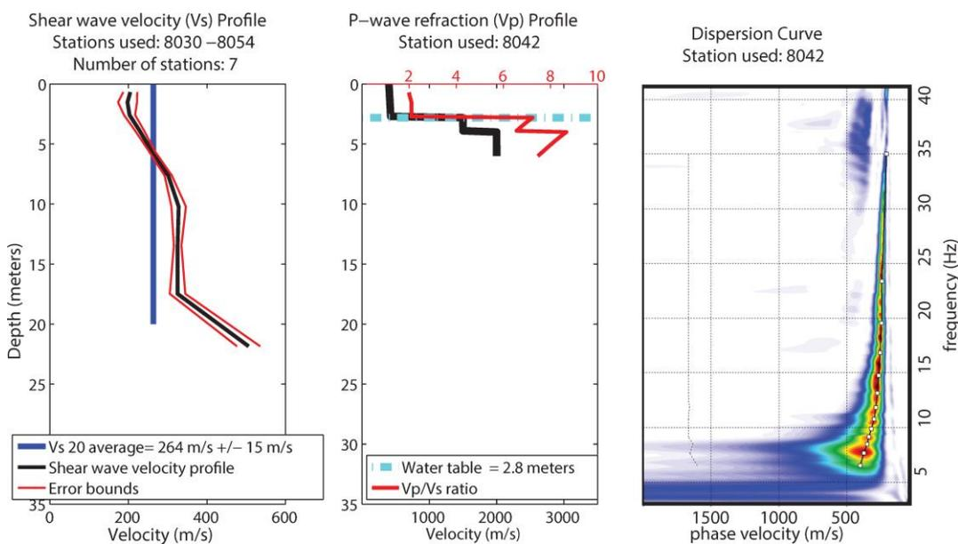
**Figure 19. (left) Shear wave velocity profile and average VS30 calculation for the central portion of the Second Street profile. (middle) P-wave, Vp/Vs ratio and water table depth measurement for the central portion of the profile. (right) Shot gather derived dispersion curve and phase velocity picks suggesting high confidence results for the upper 25 m.**
