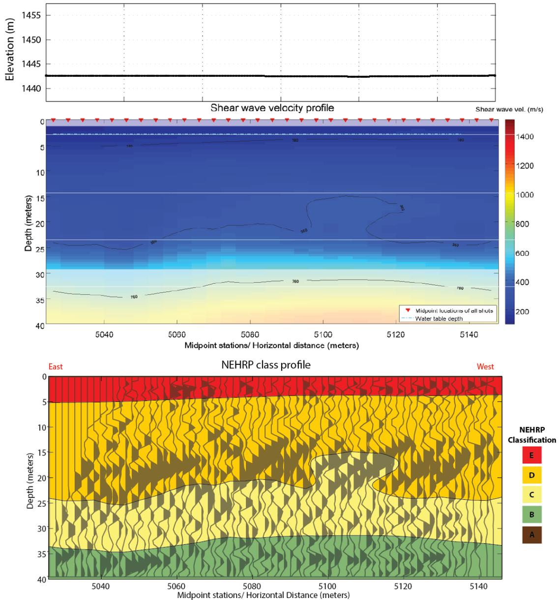
Figure 47. (top) Elevation profile for the Sewage pond access road profile. (middle) Shear wave velocity profile derived from phase velocity picks. Measurement locations are show as red triangles at the top of the plot. Semi-transparent area represents low confidence zones. (bottom) NEHRP class profile with superposition of reflection image. Velocity profile vertical exaggeration ~1:1.
