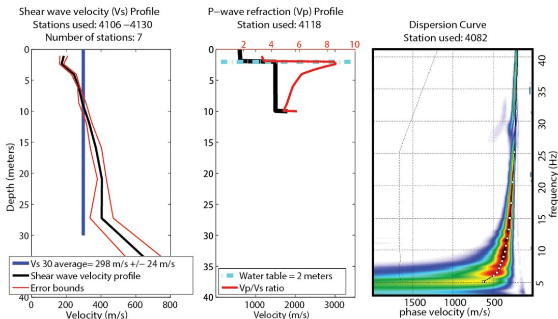
**Figure 11.** (left) Shear wave velocity profile and average Vs30 calculation for the central portion of the Lenora Street profile. (middle) P-wave, Vp/Vs ratio and water table depth measurement for the central portion of the profile. (right) Shot gather derived dispersion curve and phase velocity picks suggesting high confidence results for the upper 35 m.
