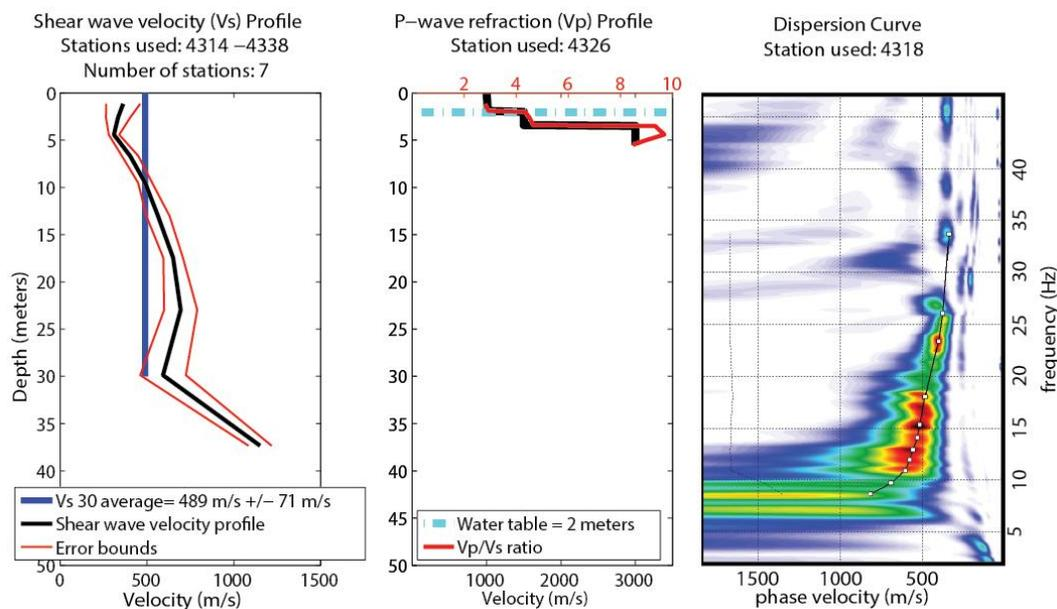
**Figure 44.** (left) Shear wave velocity profile and average VS30 calculation for the central portion of the Front Street profile. (middle) P-wave,  $V_p/V_s$  ratio and water table depth measurement for the central portion of the profile. (right) Shot gather derived dispersion curve and phase velocity picks suggesting high confidence results for the upper 38 m.
