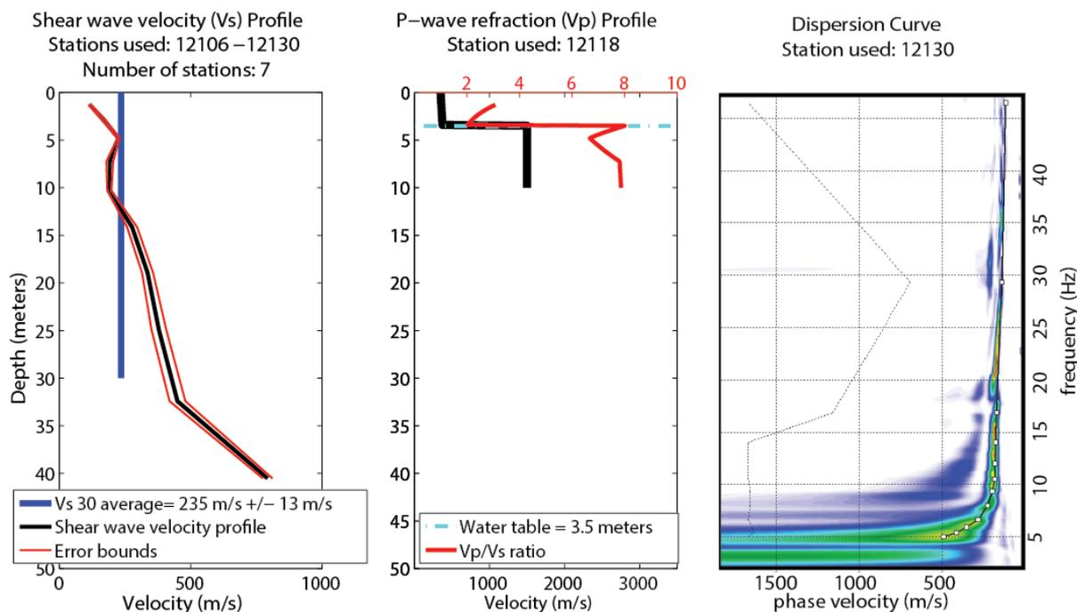
**Figure 31. (left) Shear wave velocity profile and average VS30 calculation for the central portion of the Gestrin Street profile. (middle) P-wave, Vp/Vs ratio and water table depth measurement for the central portion of the profile. (right) Shot gather derived dispersion curve and phase velocity picks suggesting high confidence results for the upper 32 m.**
