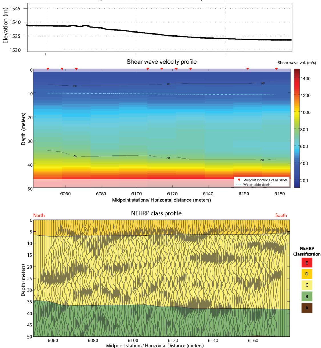
**Figure 16. (top) Elevation profile for the Thula Street profile. (middle) Shear wave velocity profile derived from phase velocity picks. Measurement locations are show as red triangles at the top of the plot. Semi-transparent area represents low confidence zones. (bottom) NEHRP class profile with superposition of reflection image. Velocity profile vertical exaggeration ~1:1.**
