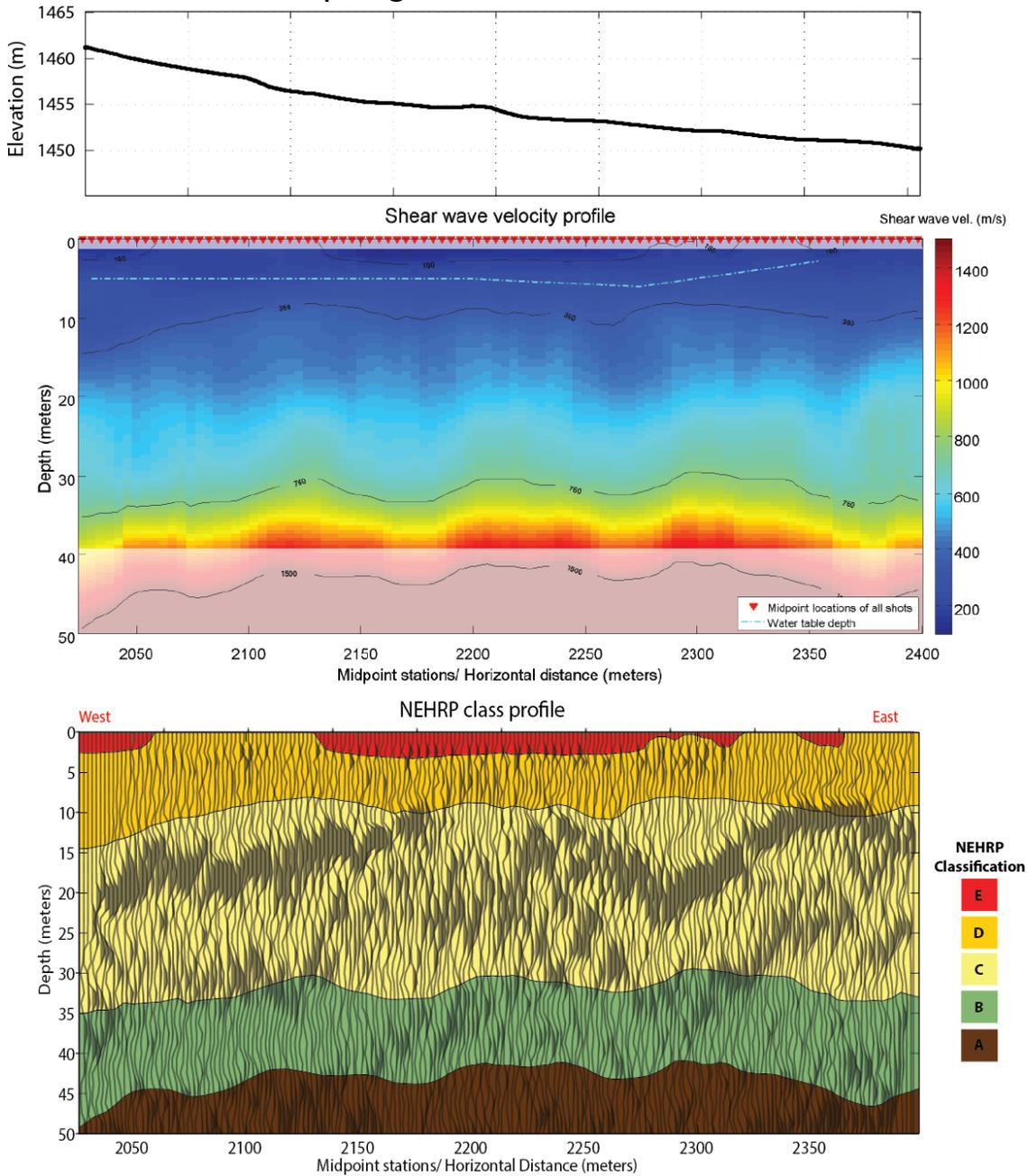
Figure 41. (top) Elevation profile for the Spring Street profile. (middle) Shear wave velocity profile derived from phase velocity picks. Measurement locations are shown as red triangles at the top of the plot. Semi-transparent areas represent low confidence zones. (bottom) NEHRP class profile with superposition of reflection image. Velocity profile vertical exaggeration ~3:1.
