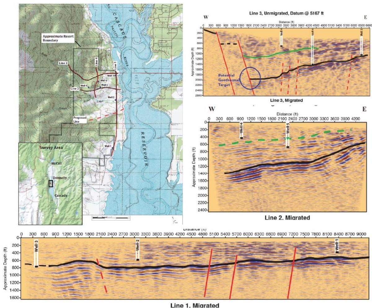
**Figure 53. Seismic images and map for the 2004 Tamarack seismic project (Bradford et al., 2004). Our results show a west-dipping bedrock surface that is truncated by the southern segment of the Long Valley fault (Personious and Lewis, 2010). The north to south Line 1 profile (bottom) suggests that bedrock deepens to the north and that west-east faults may segment Long Valley. Seismic profile vertical exaggeration ~1:1.**
