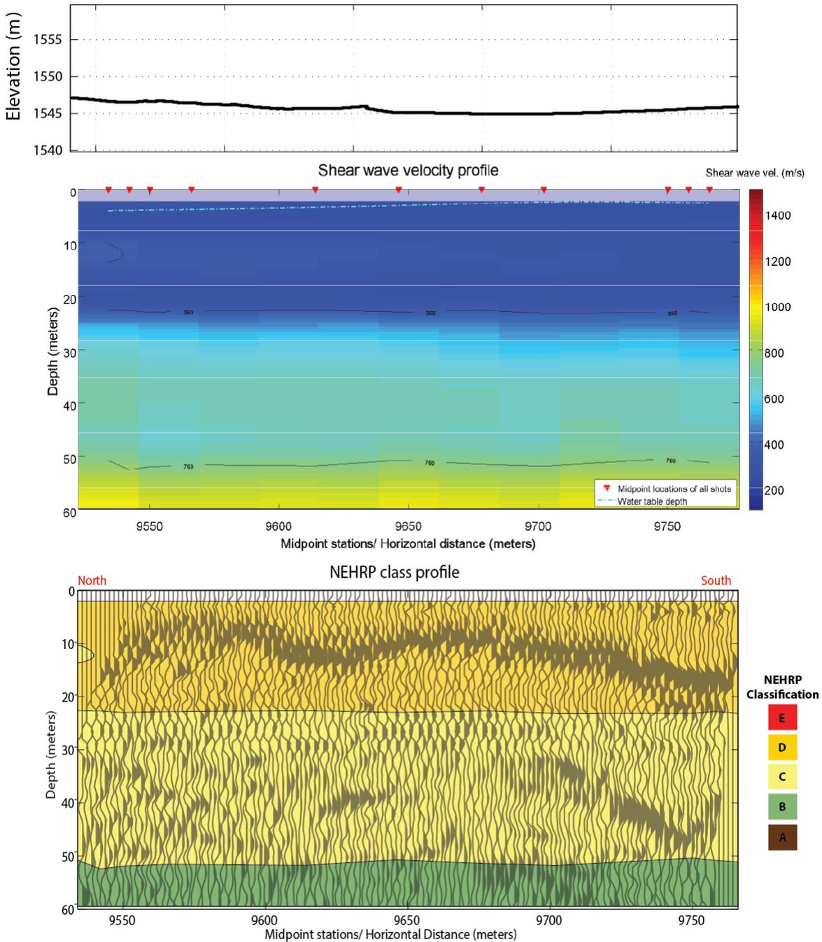
**Figure 24. (top) Elevation profile for the Samson Trail profile. (middle) Shear wave velocity profile derived from phase velocity picks. Measurement locations are show as red triangles at the top of the plot. Semi-transparent area represents low confidence zones. (bottom) NEHRP class profile with superposition of reflection image. Velocity profile vertical exaggeration ~2:1.**
