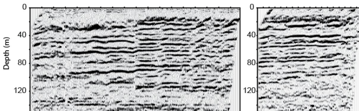
**Figure 27. Donnelly reflection profiles from Front Street & Gestrin/Halferty Roads derived from the seismic land streamer. High quality reflection data result from sedimentary layers.**
