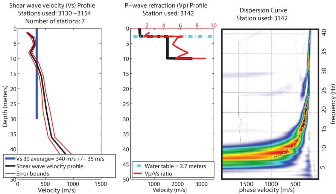
**Figure 9. (left) Shear wave velocity profile and average Vs30 calculation for the central portion of the First Street profile. (middle) P-wave, Vp/Vs ratio and water table depth measurement for the central portion of the profile. (right) Shot gather derived dispersion curve and phase velocity picks suggesting high confidence results for the upper 45 m.**
