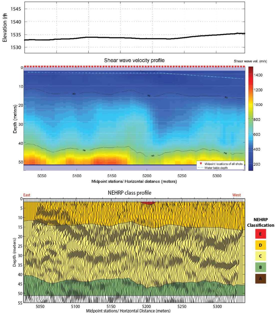
**Figure 14.** (top) Elevation profile for the Idaho Street profile. (middle) Shear wave velocity profile derived from phase velocity picks. Measurement locations are show as red triangles at the top of the plot. Semi-transparent area represents low confidence zones. (bottom) NEHRP class profile with superposition of reflection image. Velocity profile vertical exaggeration ~3:1.
