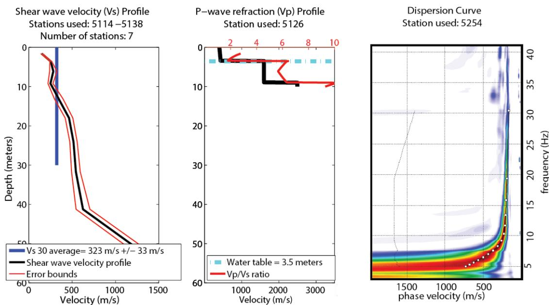
**Figure 13.** (left) Shear wave velocity profile and average VS30 calculation for the central portion of the Idaho Street profile. (middle) P-wave,  $V_p/V_s$  ratio and water table depth measurement for the central portion of the profile. (right) Shot gather derived dispersion curve and phase velocity picks suggesting high confidence results for the upper 52 m.
