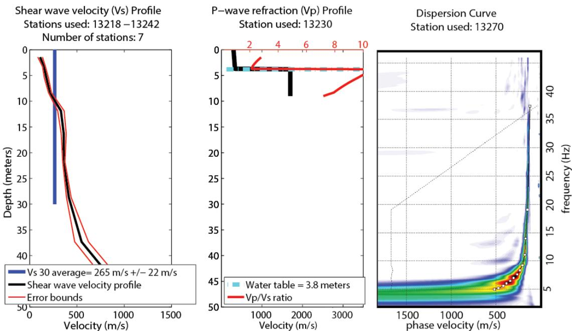
**Figure 34.** (left) Shear wave velocity profile and average  $V_{S30}$  calculation for the central portion of the Eld Street profile. (middle) P-wave,  $V_p/V_s$  ratio and water table depth measurement for the central portion of the profile. (right) Shot gather derived dispersion curve and phase velocity picks suggesting high confidence results for the upper 48 m.
