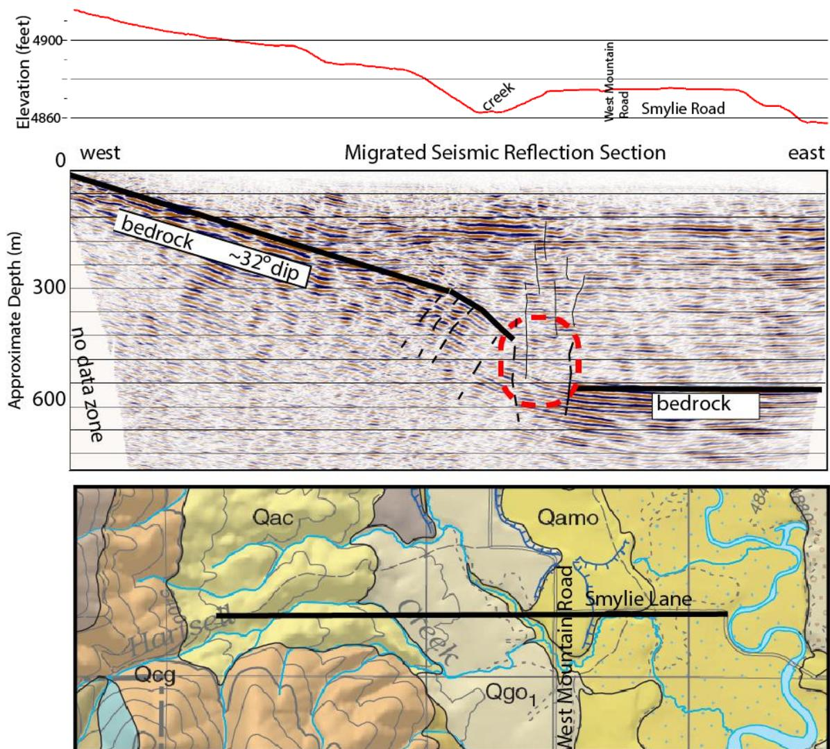
Figure 52. Smylie Road seismic reflection profile, elevation profile, and geologic map (from Breckenridge and Othberg, 2006). The profile location is shown on Figure 2 and our analysis shows a transition from a steeply dipping bedrock surface to a flat surface. The depth to bedrock is approximately 600 m along the eastern portion of the profile. Seismic profile vertical exaggeration ~2:1.
