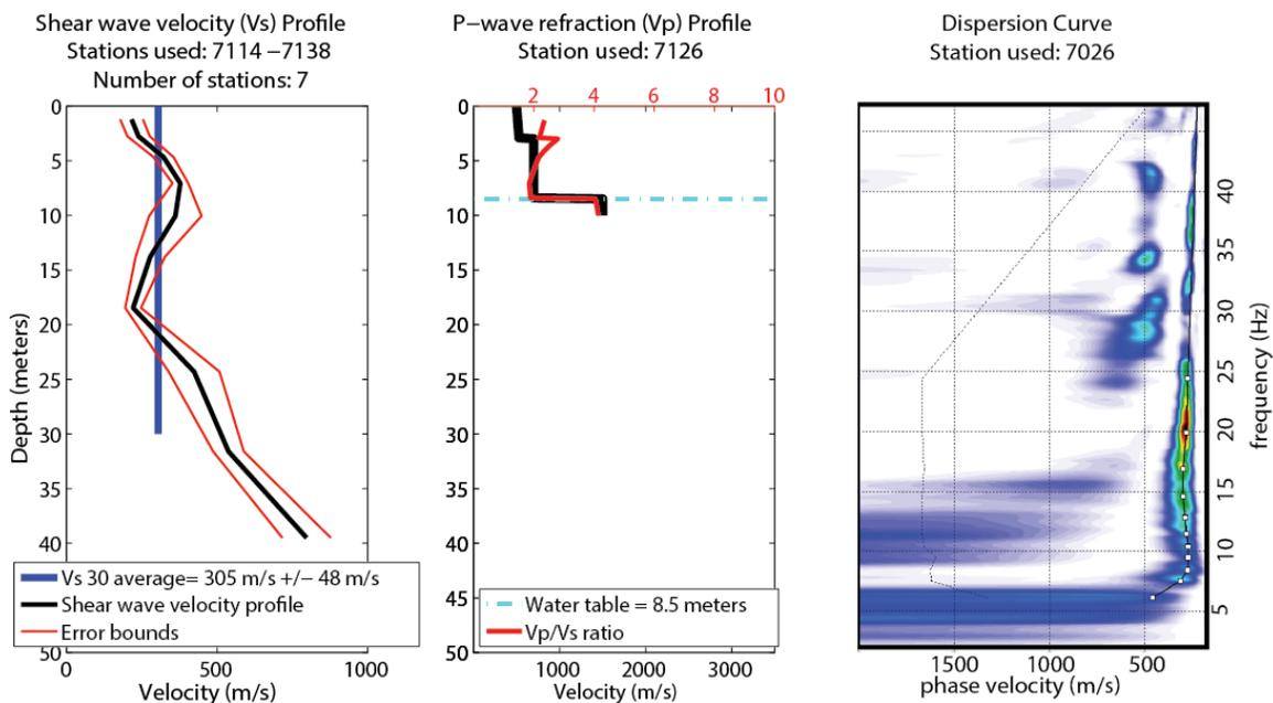
**Figure 17. (left) Shear wave velocity profile and average VS30 calculation for the central portion of the Sewage Pond profile. (middle) P-wave, Vp/Vs ratio and water table depth measurement for the central portion of the profile. (right) Shot gather derived dispersion curve and phase velocity picks suggesting high confidence results for the upper 40 m.**
