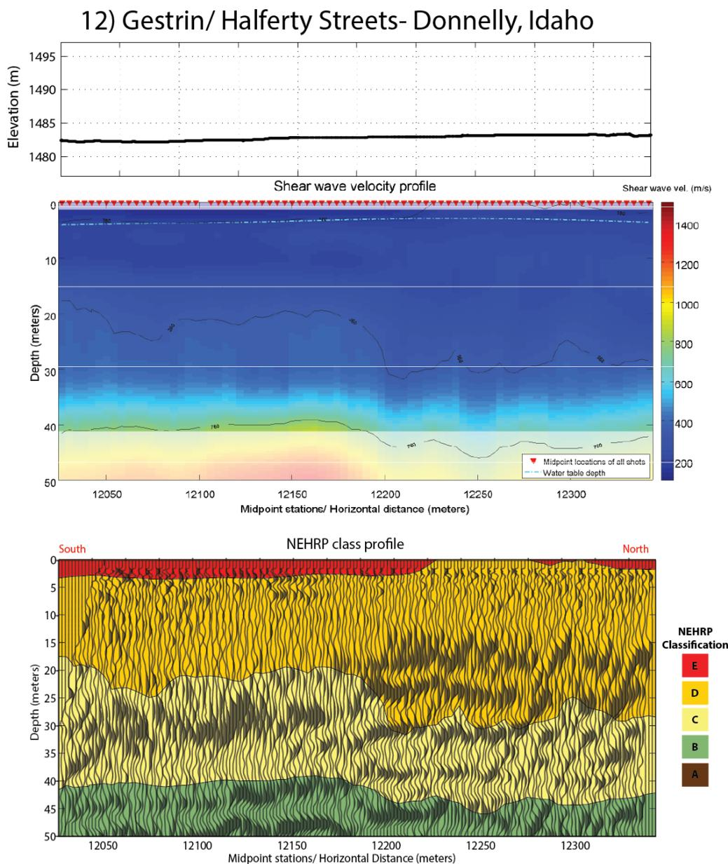
Figure 32. (top) Elevation profile for Halferty/Gestrin Street profile. (middle) Shear wave profile derived from phase velocity picks. Measurement locations are show as red triangles at the top of the plot. Semi-transparent area represents low confidence zones. (bottom) NEHRP class profile with superposition of reflection image. Velocity profile vertical exaggeration ~3:1.
