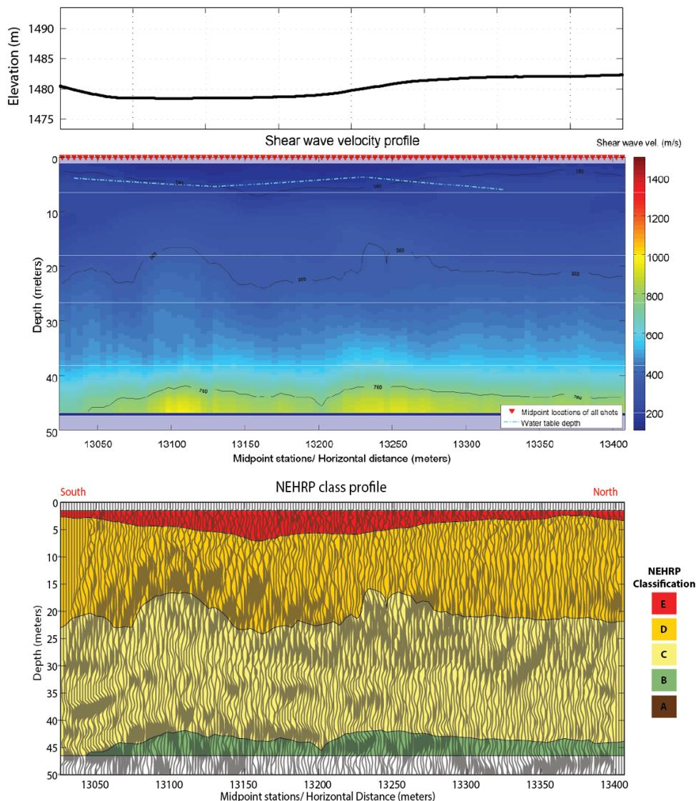
Figure 35. (top) Elevation profile for the Eld Street profile, sewage pond access road. (middle) Shear wave velocity profile derived from phase velocity picks. Measurement locations are show as red triangles at the top of the plot. Semi-transparent area represents low confidence zones. (bottom) NEHRP class profile with superposition of reflection image. Velocity profile vertical exaggeration ~3:1.
