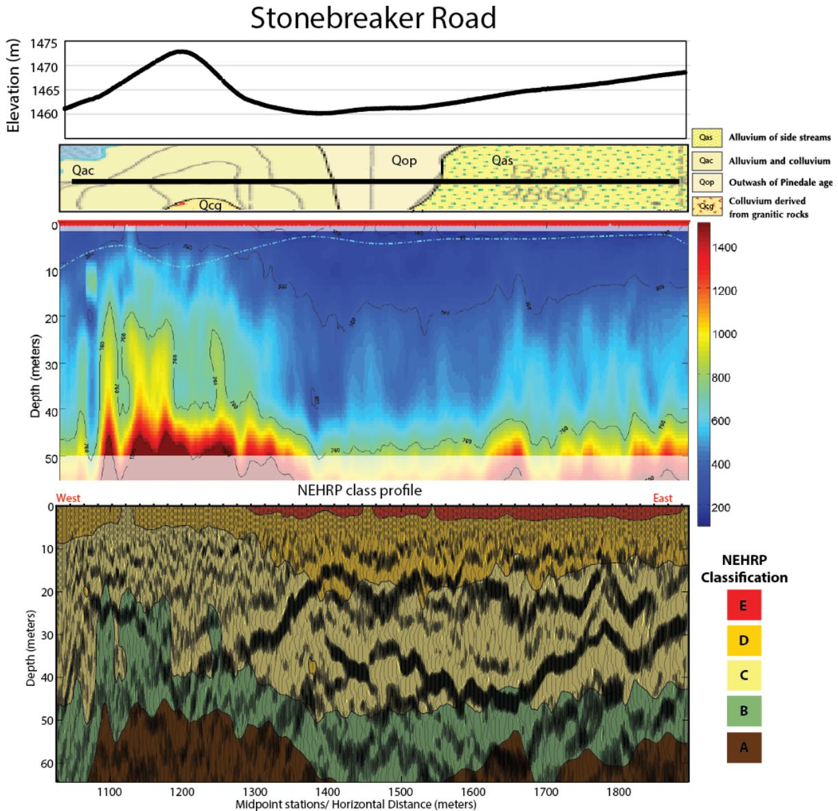
**Figure 51. (top) Elevation profile for the Stonebreaker Road profile. (middle) Shear wave velocity profile derived from phase velocity picks. Measurement locations are show as red triangles at the top of the plot. Semi-transparent area represents low confidence zones. (bottom) NEHRP class profile with superposition of reflection image. Velocity profile vertical exaggeration ~5:1.**
