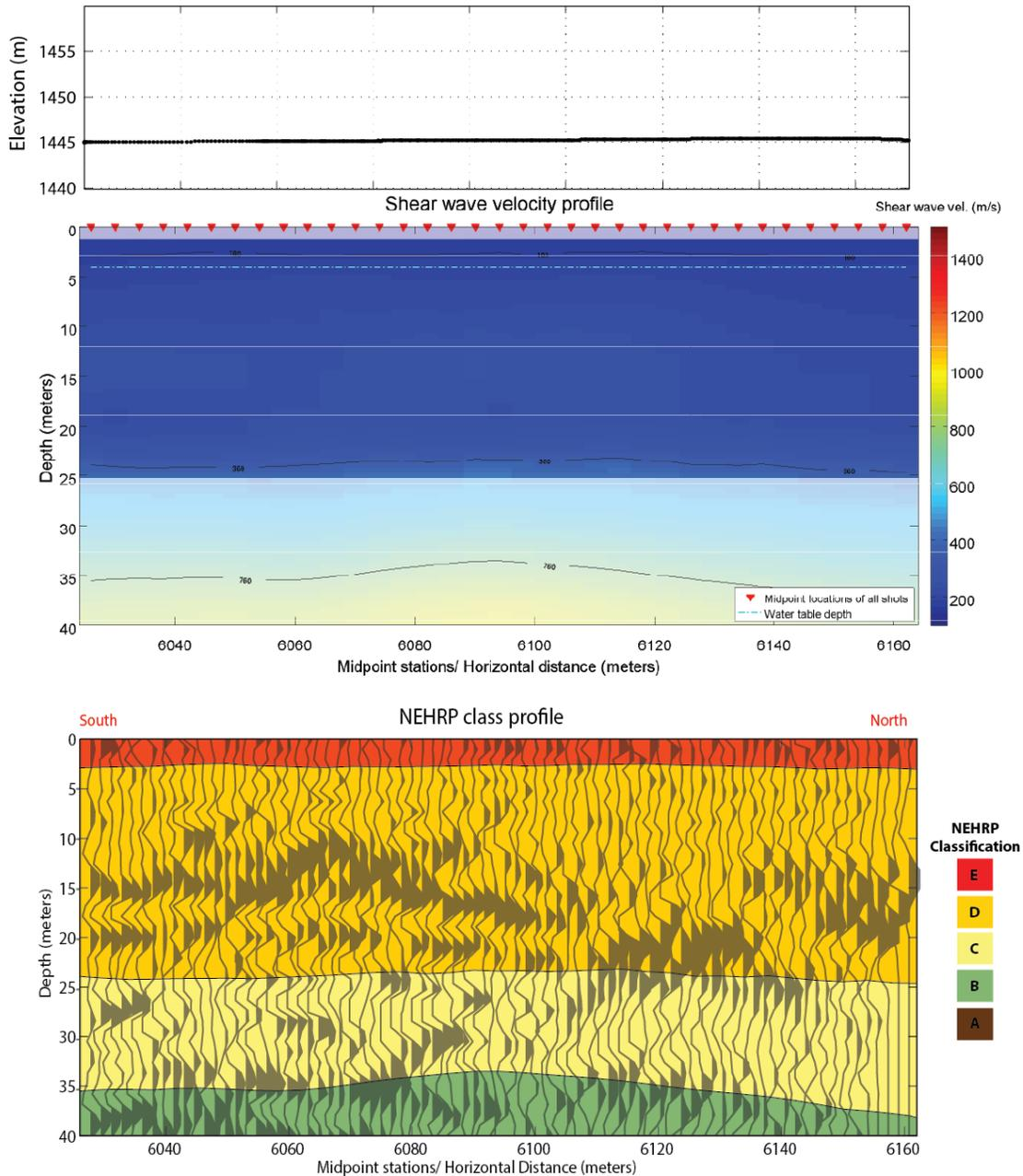
Figure 49. (top) Elevation profile for the Alzar Street profile. (middle) Shear wave velocity profile derived from phase velocity picks. Measurement locations are show as red triangles at the top of the plot. Semi-transparent area represents low confidence zones. (bottom) NEHRP class profile with superposition of reflection image. Velocity profile vertical exaggeration ~1.5:1.
