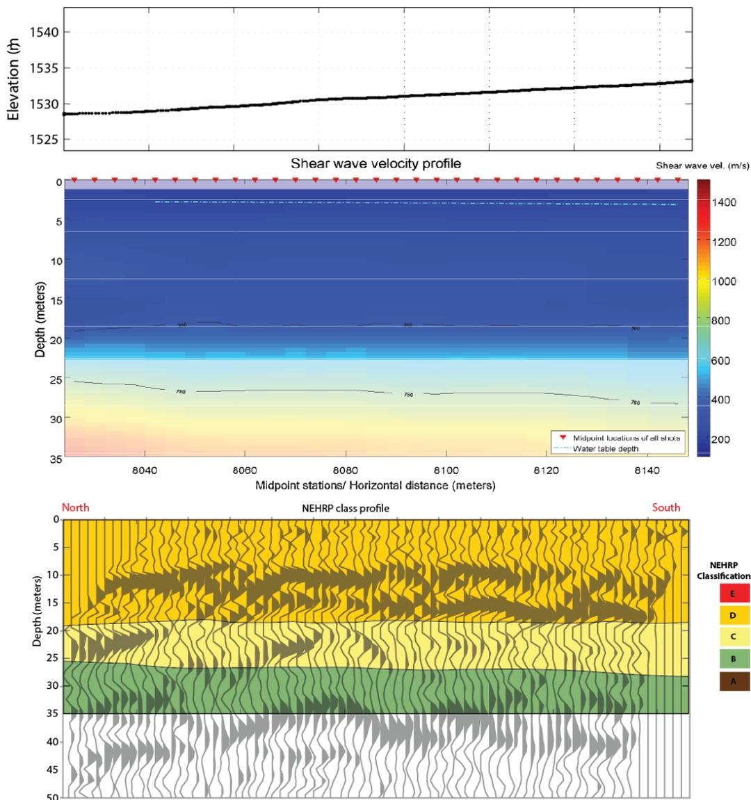
**Figure 20. (top) Elevation profile for the Second Street profile. (middle) Shear wave velocity profile derived from phase velocity picks. Measurement locations are show as red triangles at the top of the plot. Semi-transparent area represents low confidence zones. (bottom) NEHRP class profile with superposition of reflection image. Velocity profile vertical exaggeration ~1:1.**
