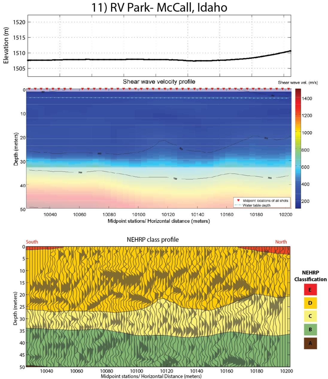
Figure 26. (top) Elevation profile for the RV Park access road profile. (middle) Shear wave velocity profile derived from phase velocity picks. Measurement locations are show as red triangles at the top of the plot. Semi-transparent area represents low confidence zones. (bottom) NEHRP class profile with superposition of reflection image. Velocity profile vertical exaggeration ~1.5:1.
