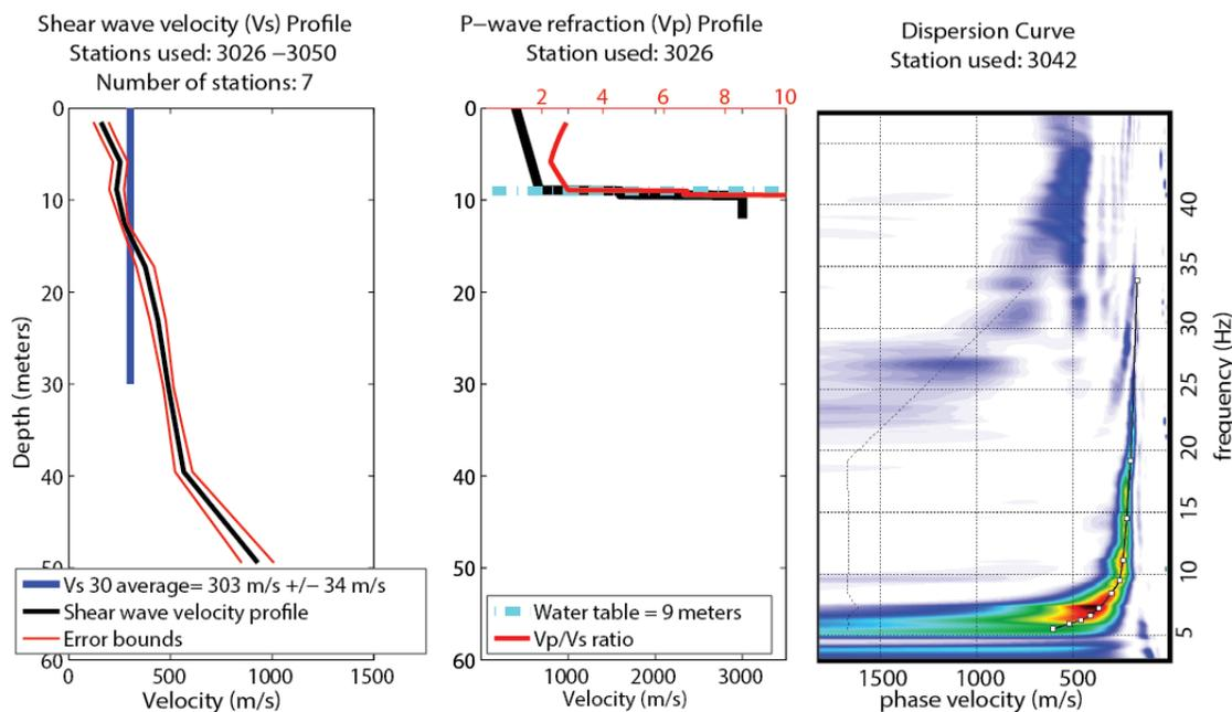
**Figure 42. (left) Shear wave velocity profile and average VS30 calculation for the Lefever Drive (Medical Center) profile. (middle) P-wave,  $V_p/V_s$  ratio and water table depth measurement for the central portion of the profile. (right) Shot gather derived dispersion curve and phase velocity picks suggesting high confidence results for the upper 49 m.**
