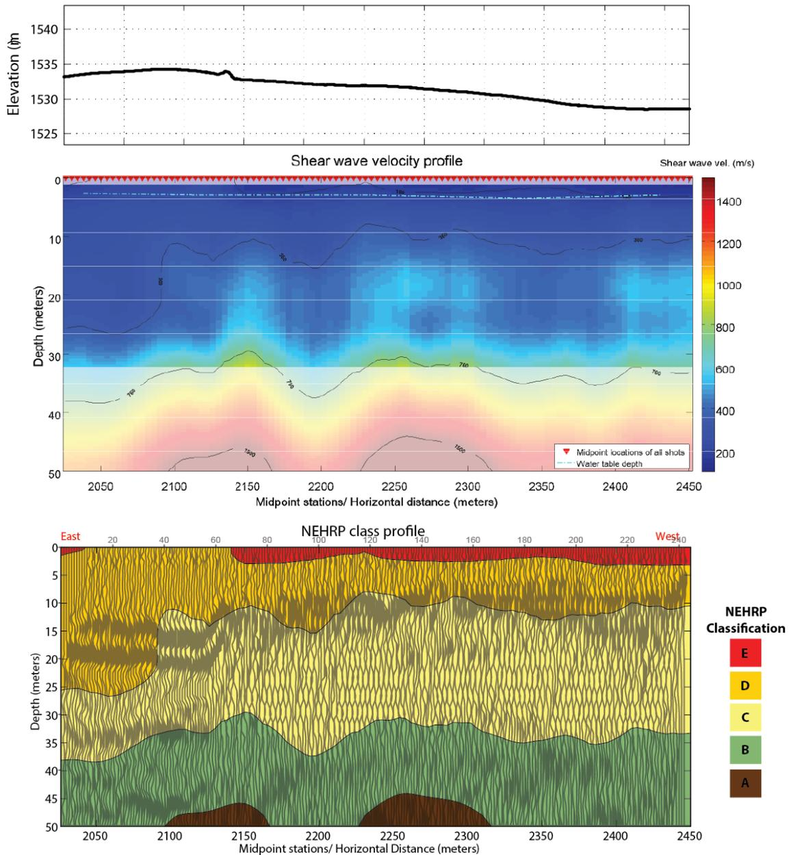
Figure 7. (top) Elevation profile for the Park Street profile. (middle) Shear wave velocity profile derived from phase velocity picks. Measurement locations are show as red triangles at the top of the plot. Semi-transparent area represents low confidence zones. (bottom) NEHRP class profile with superposition of reflection image. Velocity profile vertical exaggeration ~4:1.
