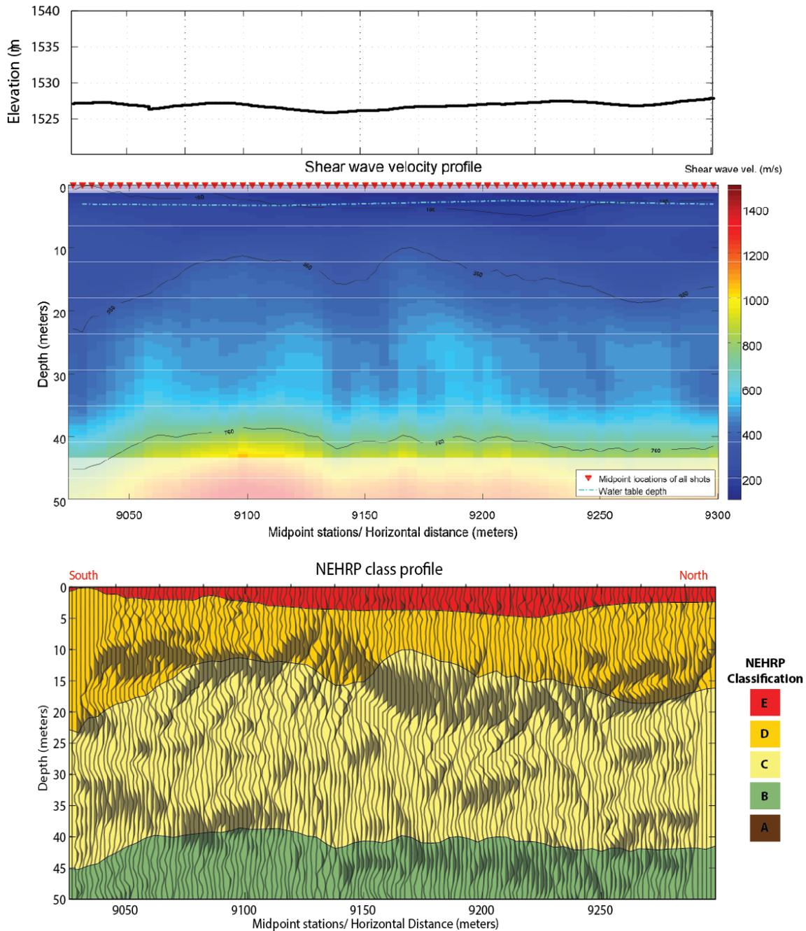
Figure 22. (top) Elevation profile for the Mill Street profile. (middle) Shear wave velocity profile derived from phase velocity picks. Measurement locations are show as red triangles at the top of the plot. Semi-transparent area represents low confidence zones. (bottom) NEHRP class profile with superposition of reflection image. Velocity profile vertical exaggeration ~2.5:1.
