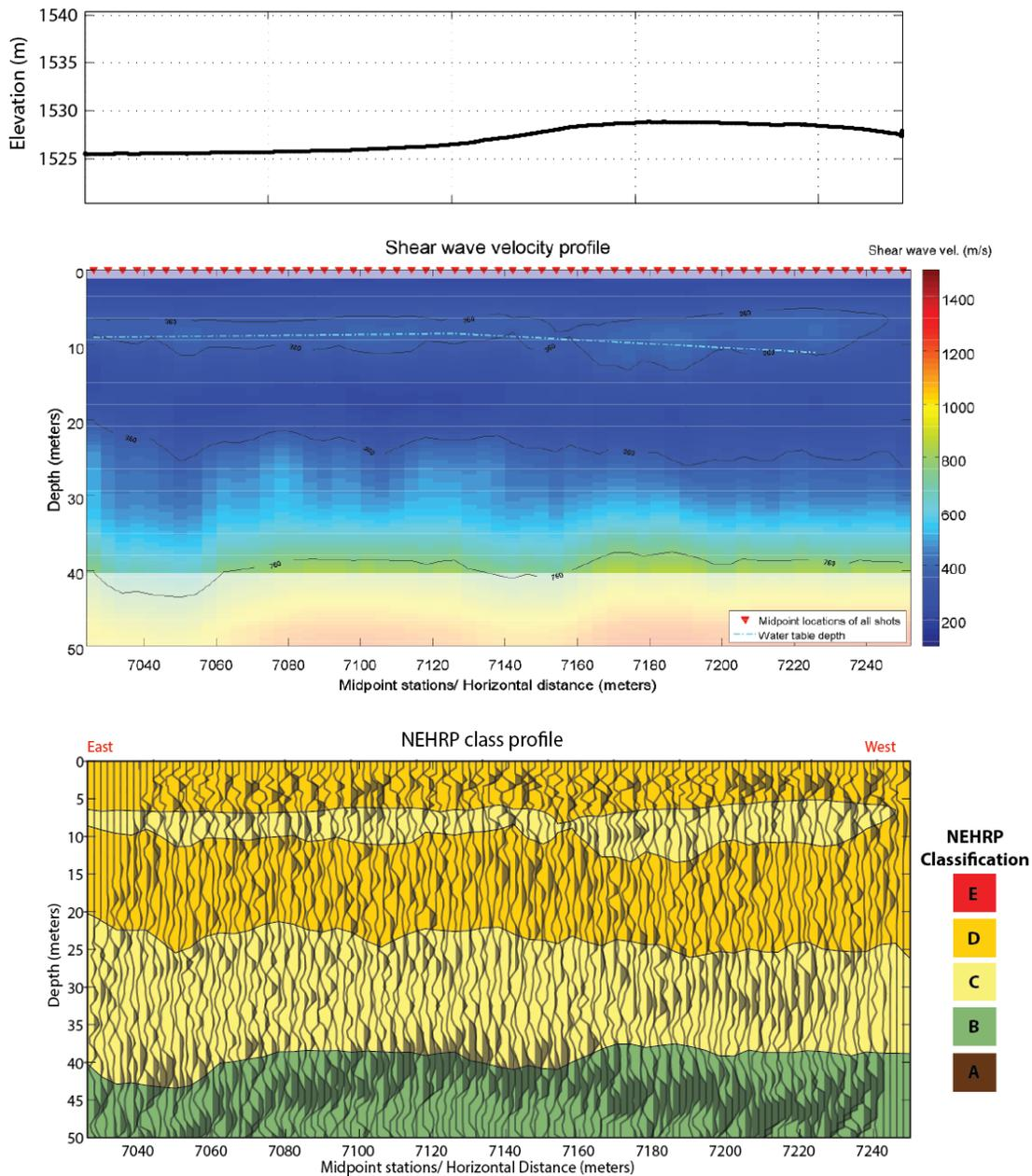
Figure 18. (top) Elevation profile for the Sewage Ponds profile. (middle) Shear wave velocity profile derived from phase velocity picks. Measurement locations are show as red triangles at the top of the plot. Semi-transparent area represents low confidence zones. (bottom) NEHRP class profile with superposition of reflection image. Velocity profile vertical exaggeration ~2:1.
