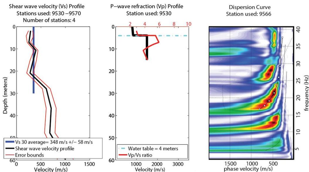
**Figure 23.** (left) Shear wave velocity profile and average Vs30 calculation for the central portion of the South Samson Trail Road profile. (middle) P-wave, Vp/Vs ratio and water table depth measurement for the central portion of the profile. (right) Shot gather derived dispersion curve and phase velocity picks suggesting high confidence results for the upper 60 m.
