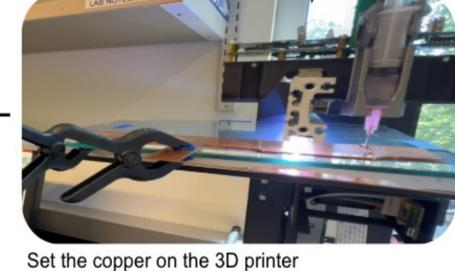
Set the copper on the 3D printer
