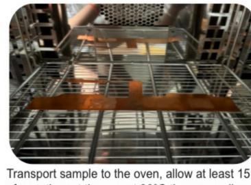
Transport sample to the oven, allow at least 15 minutes of cure time at the preset 90°C, then annealing at 130°C for 1 hours
