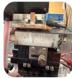
Use corona poling polarization the sample at 40°C, 60°C and 80°C
