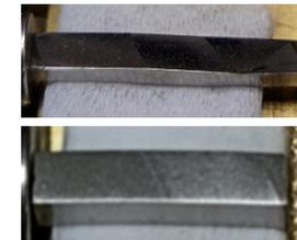
*Twinning Comparison: Polished (top), Micropeened (bottom)*
