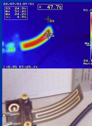
Closed sample heated with 1.2 amps for three minutes
