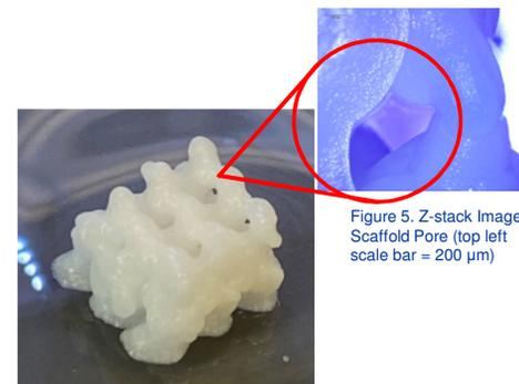
Figure 4. 3D Printed Bone Scaffold
