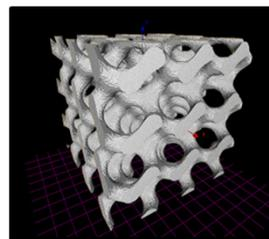
Figure 2. Trabecular Bone Gyroid Structure .stl File
