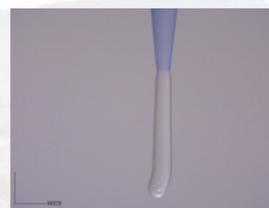
Figure 3. Bioink Filament Test (2mm scale bar)
