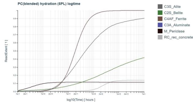
Figure 4.2: Plot containing the hydration reaction extent of clinker phases (alite, belite, ferrite, aluminate) and the extent of the recycled concrete fines. Up to 15% of the RCF is able to react to form hydration products.
