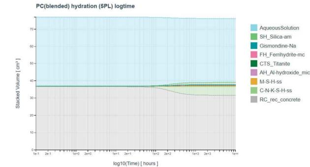
Figure 4.1: Stacked volume plot for 100g RCF & 0.4 w/b ratio
