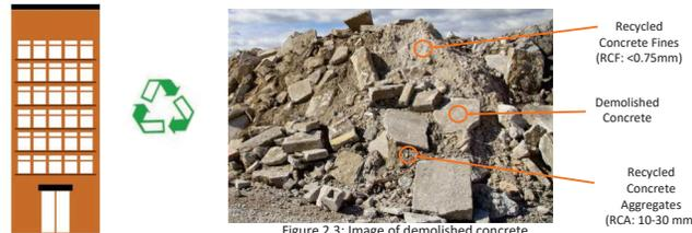
Figure 2.3: Image of demolished concrete
