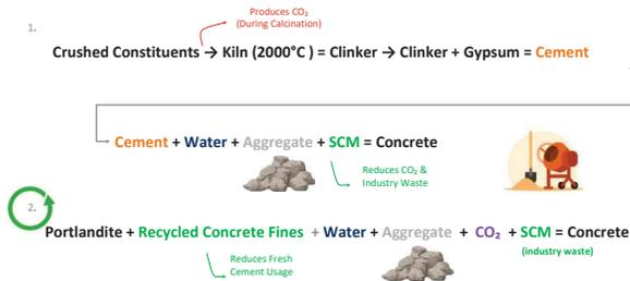
Figure 1.2 : Comparison of current concrete production process (1) with novel concrete process (2)
