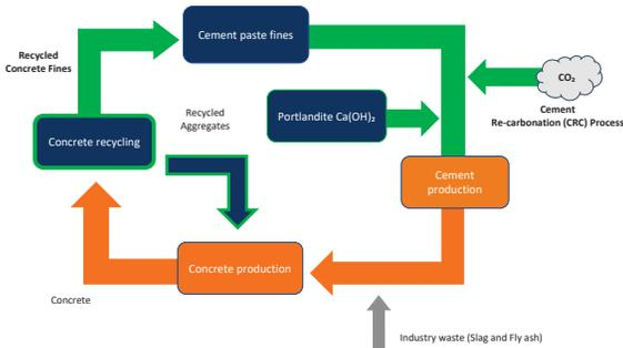
Figure 1.1: Concrete life cycle with lower CO<sub>2</sub> emissions. The green coloring represents the cycle improvements on the original orange process.
