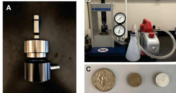
**Figure 4.** Coated powder was pressed with aqueous  $\text{Li}_2\text{MoO}_4$  at 650 MPa under vacuum. **A.** Vacuum die. **B.** Uniaxial pellet press with vacuum pump. **C.** Pellet and silver-coated pellet relative to a nickel (from right to left).
