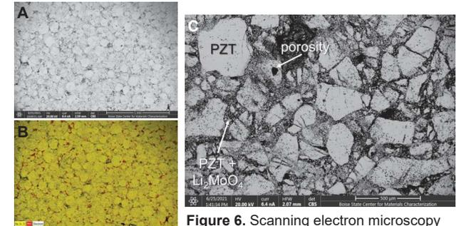
**Figure 6.** Scanning electron microscopy images of ceramic composites. **A.** Backscattered electron image of  $\text{Ba}_{0.5}\text{Sr}_{0.5}\text{TiO}_3$  pellet. **B.** Phase mapping by EDS analysis of the same location, with yellow corresponding to BST, red to  $\text{Li}_2\text{MoO}_4$ , and black to porosity. **C.** Backscattered electron image of  $\text{PbZr}_{0.5}\text{Ti}_{0.5}\text{O}_3$  pellet, with phases labelled.
