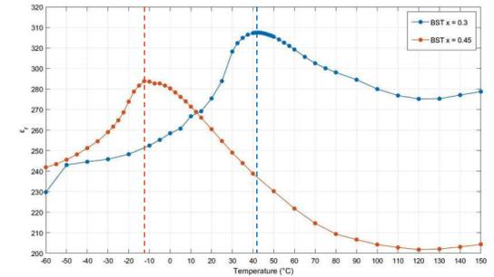
**Figure 5.** Dielectric properties of BST composites as a function of temperature at 1 kHz while cooling. In both cases, the Curie temperature ( $T_c$ ) is indicated by a vertical dashed line.
