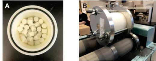
**Figure 1.** Stoichiometric  $\text{PbO}$ ,  $\text{ZrO}_2$ ,  $\text{TiO}_2$  powders were milled. **A.** Mill pot with milling media. **B.** Rotary mill.
