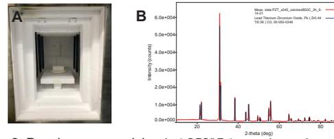
**Figure 2.** Powders were calcined at  $850^\circ\text{C}$  to produce phase-pure PZT. **A.** Covered crucible in box furnace. **B.** XRD pattern of  $\text{PbZr}_{0.5}\text{Ti}_{0.5}\text{O}_3$  (red) with reported peak locations of  $\text{PbZr}_{0.44}\text{Ti}_{0.56}\text{O}_3$  for verification (blue).
