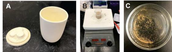
**Figure 3.** Calcined and milled powder was sintered at  $1150^\circ\text{C}$  in an inverted crucible and then coated with  $\text{Li}_2\text{MoO}_4$ . **A.** Powder pressed into pellets and coated with sacrificial powder. **B.** Coating procedure. **C.** Coated PZT.
