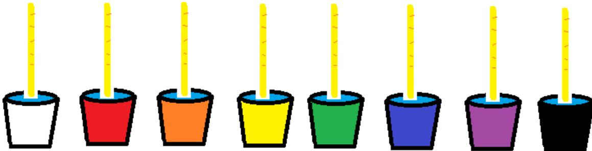
Place the cups side by side in a sunny window, or outdoors (and out of the wind) in the sun on a warm sunny day. Or, the thermometers can be placed side by side under a pair of heat lamps.
