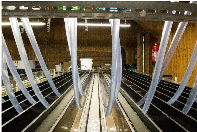
Figure 4.8. Downstream view of flume. Flume and tile width are 5 cm. Tubes connect effluent and influent reservoirs. One tube delivered effluent water to influent reservoir, and the second tube served as overflow.
