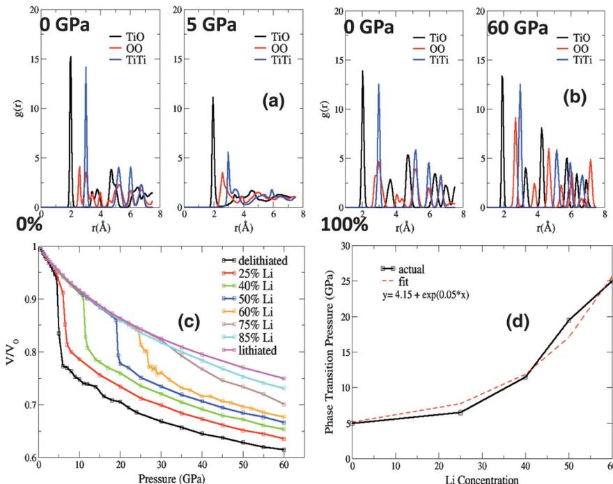
FIG. 2 (color). (a) Theoretical PRDF of the pairs for the delithiated (0%) cubic TiO<sub>2</sub> at 0 and 5 GPa. (b) PRDF of the pairs for the fully lithiated (100%) cubic TiO<sub>2</sub> at 0 and 60 GPa. (c) Volume changes as a function of the pressure for each concentration. (d) Phase transition pressure as a function of Li concentration.
