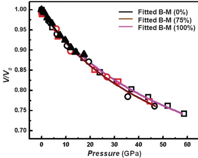
FIG. 3 (color). Relative unit cell volume changes with pressure in *c*-TiO<sub>2</sub> nanotubes with different Li concentration based on the data presented in Fig. 1. Solid lines are fitted curves by B-M EOS. Symbols: 0% solid triangles; 75% open circles; 100% open squares. Compression is shown in black, release in red. Error bars are within the symbols.
