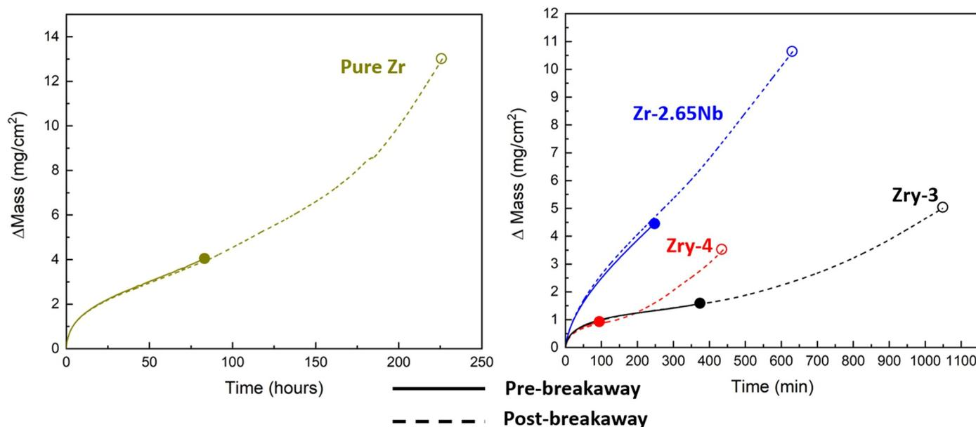
**Fig. 1.** Normalized mass gain during isothermal oxidation for zirconium in hours of exposure (left) and its alloys in minutes of exposure (right). Pre-breakaway samples are designated with solid lines, post-breakaway samples with dotted lines. End points are noted with large dots.
