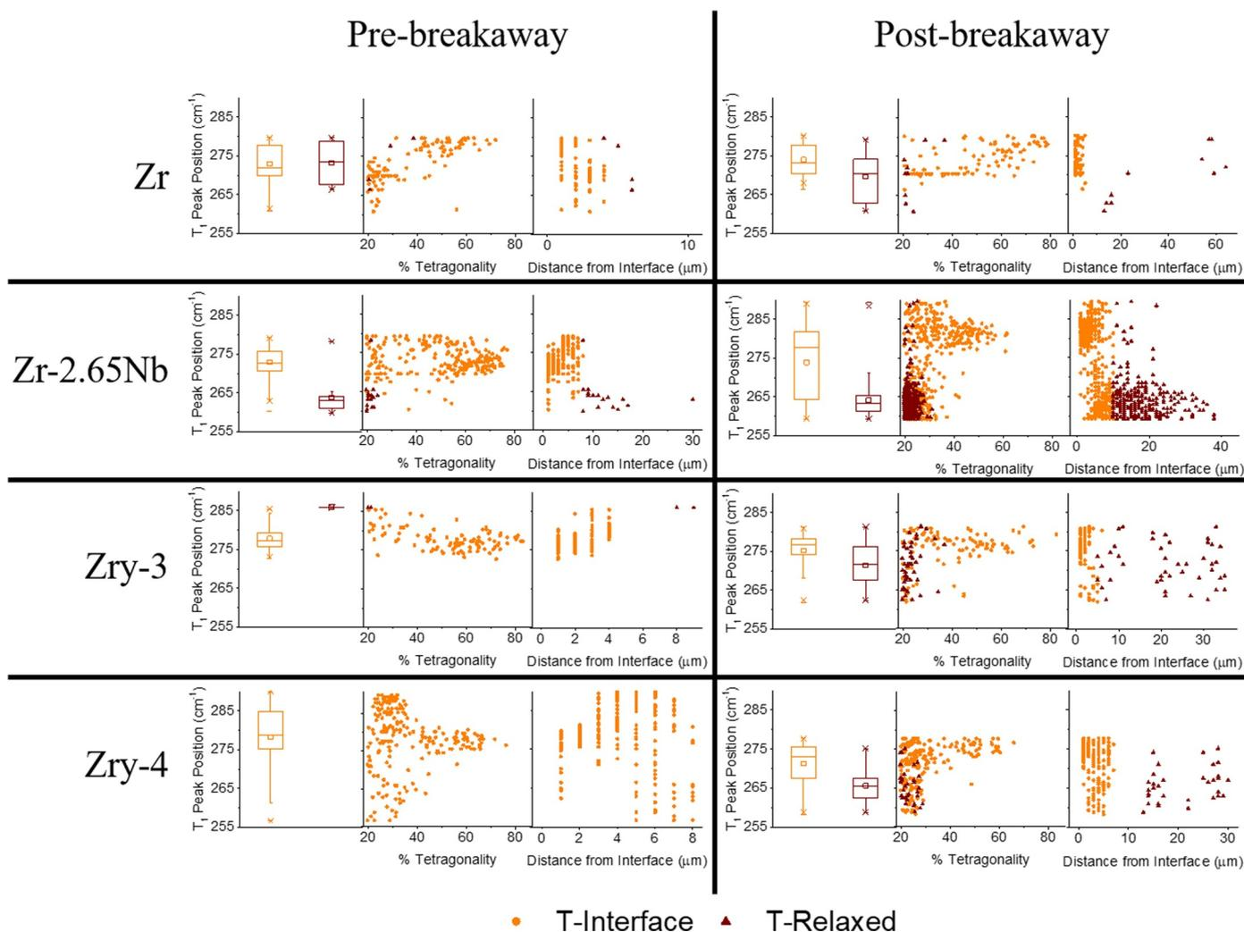
Fig. 4. Tetragonal ( $T_1$ ) peak position of tetragonal-interface and tetragonal-relaxed phases for each alloy, pre- and post-breakaway. Shown for each sample are (left) box-and-whisker plots for the  $T_1$  peak position of each tetragonal phase, (center)  $T_1$  peak position as a function of the percent tetragonality calculated for each spectrum with Eq. (1), and (right)  $T_1$  peak position as a function of distance along the horizontal axis from the metal/oxide interface.
