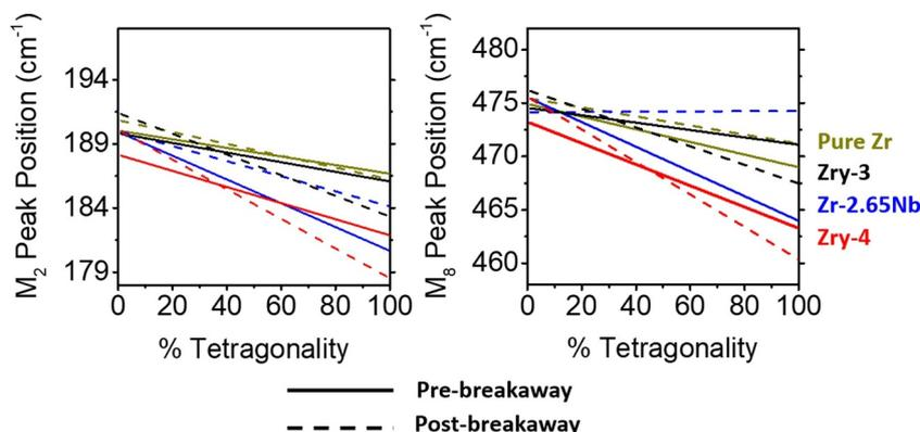
Fig. 9. Linear trends of monoclinic peak positions,  $M_2$  (left) and  $M_8$  (right), as a function of percent tetrangality. Pre-breakaway samples are designated with solid lines, post-breakaway samples with dotted lines.
