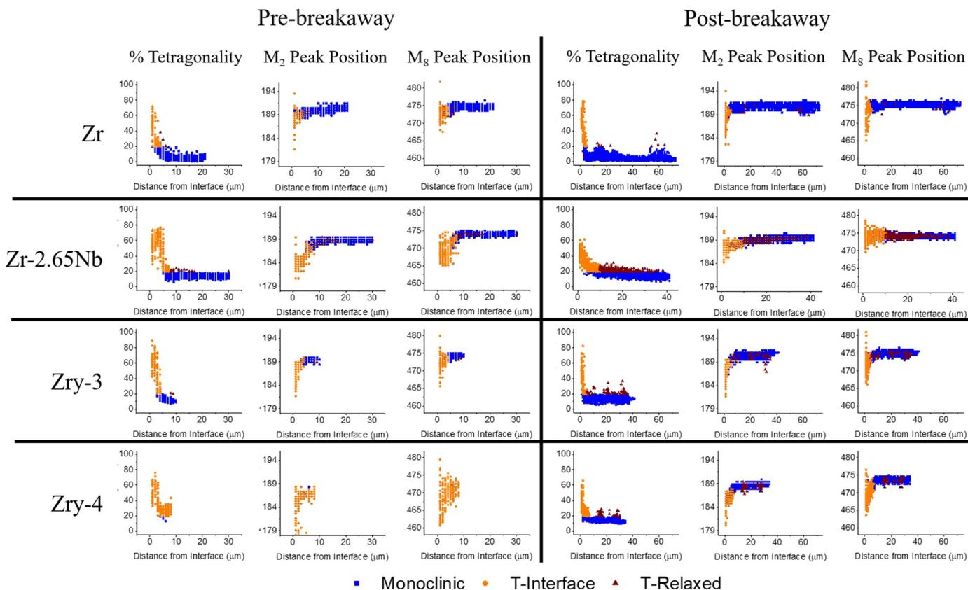
Fig. 8. Percent tetrangality and monoclinic peak positions,  $M_2$  and  $M_8$  (in  $\text{cm}^{-1}$ ), as a function of distance from the metal/oxide interface for each alloy, pre- and post-breakaway.
