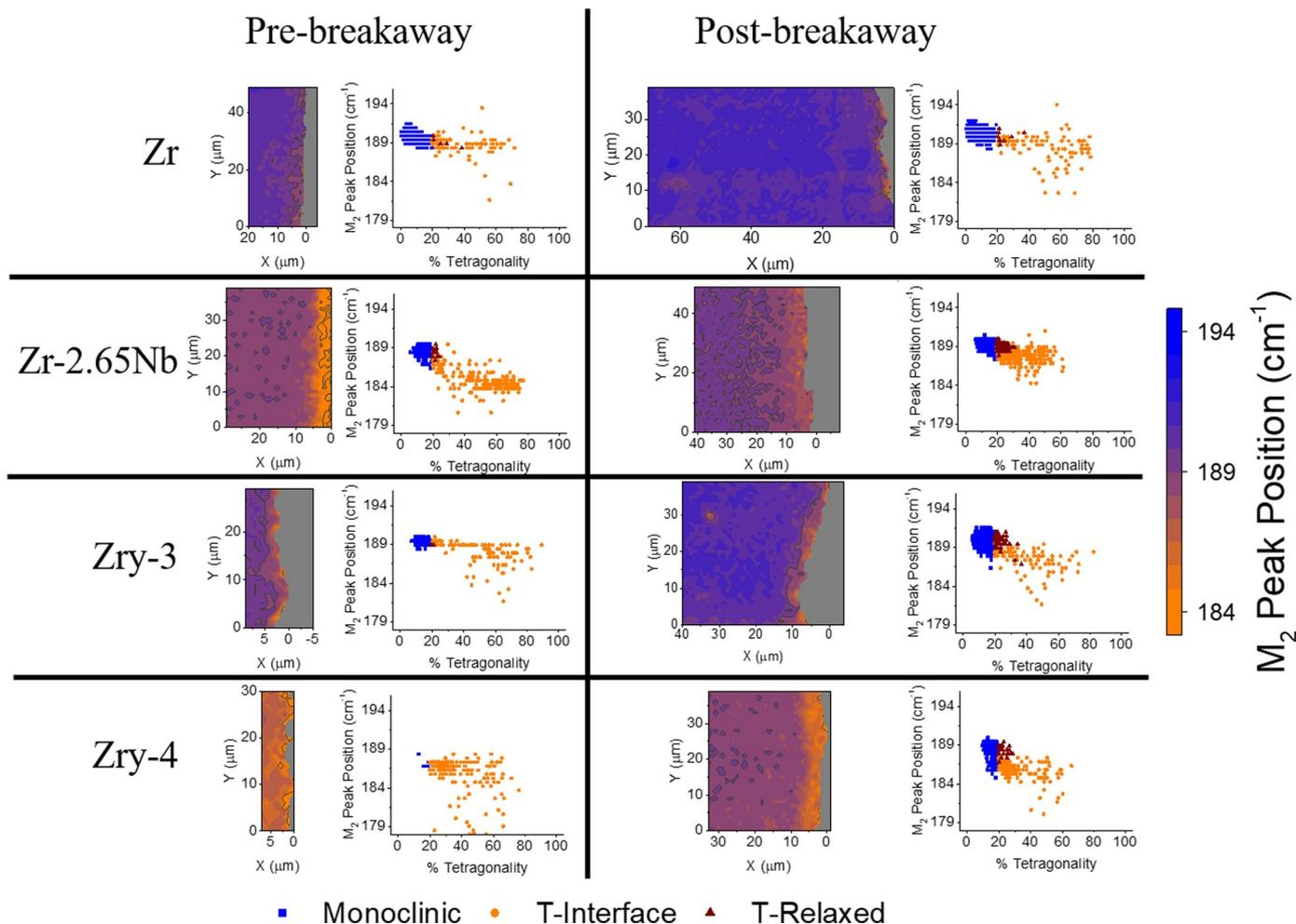
Fig. 6. Raman mapping of  $M_2$  peak position for each sample, both pre- and post-breakaway. Scatter plots of  $M_2$  peak position as a function of percent tetragonality are also included for each Raman map.
