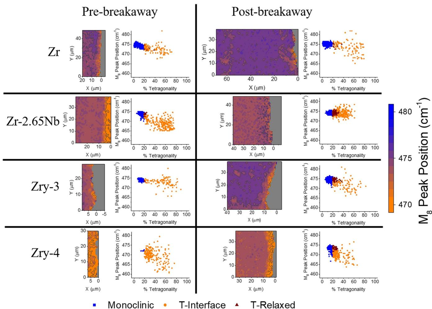
**Fig. 7.** Raman mapping of  $M_8$  peak position for each sample, both pre- and post-breakaway. Scatter plots of  $M_8$  peak position as a function of percent tetragonality are also included for each Raman map.
