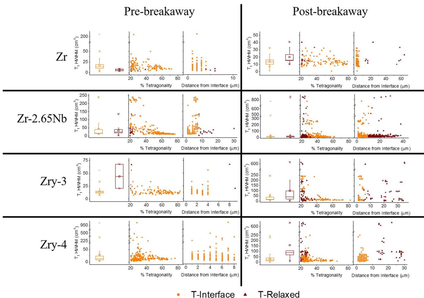
Fig. 5. Tetragonal ( $T_1$ ) HWHM of tetragonal-interface and tetragonal-relaxed phases for each alloy, pre- and post-breakaway. Shown for each sample are (left) box-and-whisker plots for the  $T_1$  HWHM of each tetragonal phase, (center)  $T_1$  HWHM as a function of the percent tetragonality calculated for each spectrum with Eq. (1), and (right)  $T_1$  HWHM as a function of distance along the horizontal axis from the metal/oxide interface.
