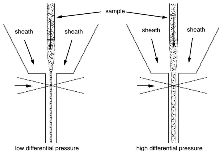
**Figure 2-2** Hydrodynamic focusing of the sample core through a nozzle tip
