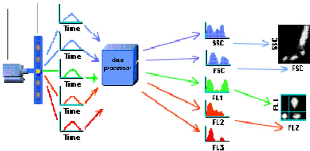
**Figure 1-1** Scattered and emitted light signals are converted to electronic pulses that can be processed by the computer
