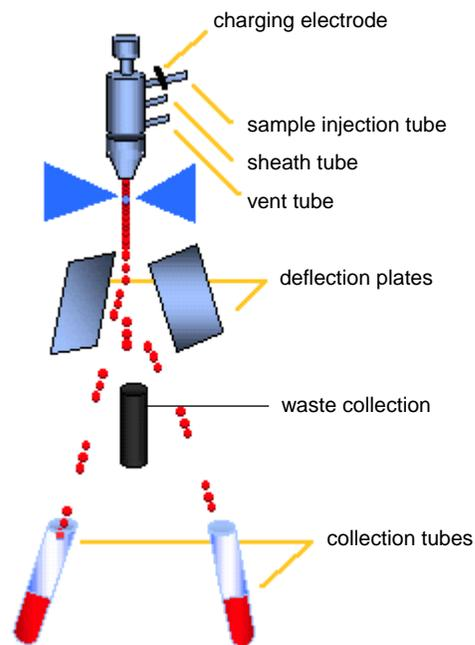
Figure 6-2 Sorting components on the FACSVantage SE
